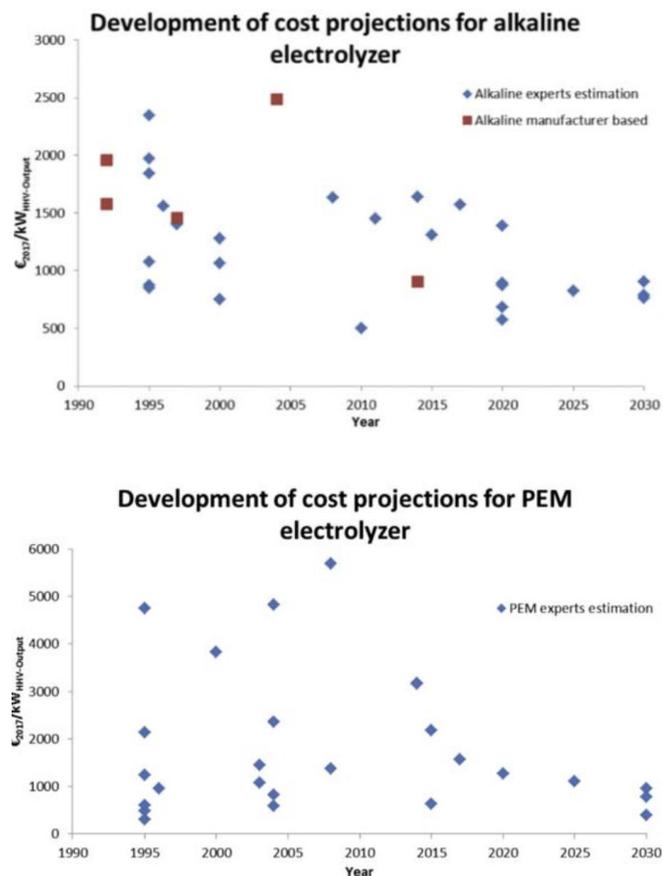
Fig. 4. CAPEX estimate for AWE and PEM technologies (source: Université catholique de Louvain)
