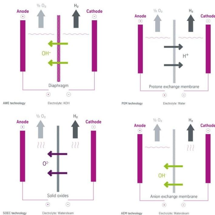
Fig. 3. **Principal schemes of electrolysis process for AWE, PEM, SOEC and AEM (source: Thyssenkrupp Nucera)**
