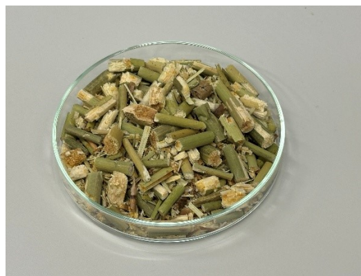
Fig. 2. Sample of chopped lake rush ( Scirpus lacustris ). The main mass consists of 1.5-3 cm long fibres, between which a finer filling can be observed
