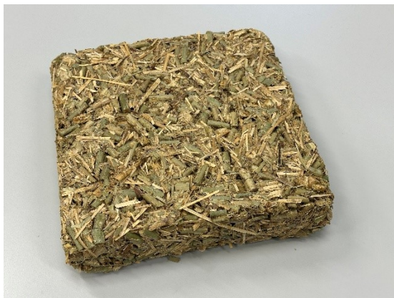
Fig. 3. Sample of the developed thermal insulation, size 20 x 20 x 5 cm. One-piece structure, reinforced with longer reed fibres
