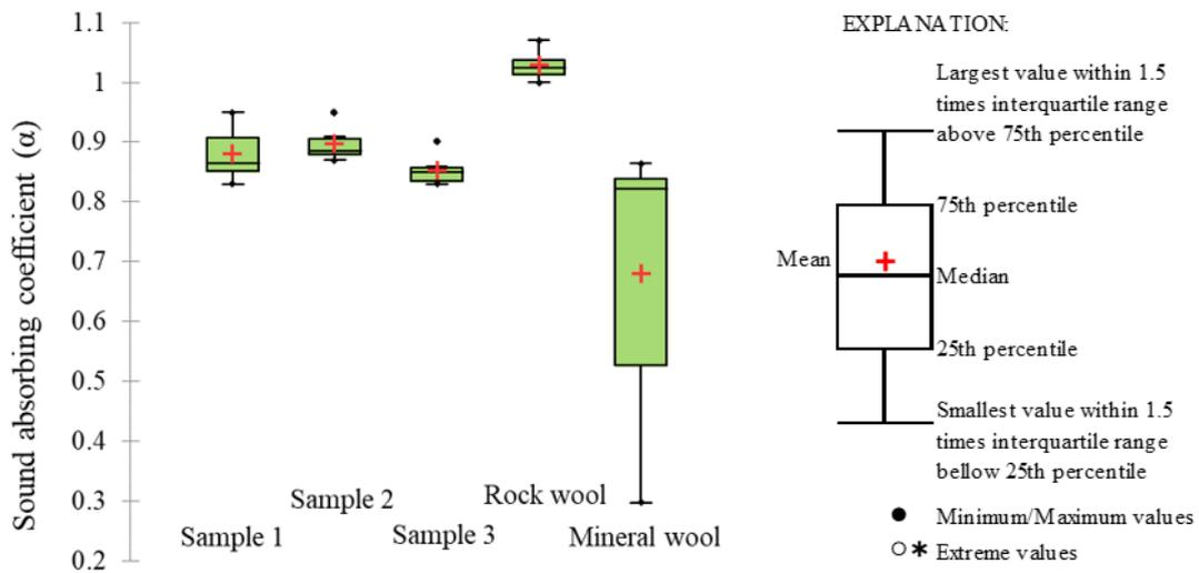
Fig. 9. Sound absorption coefficients at high frequencies (1250-4000 Hz)
