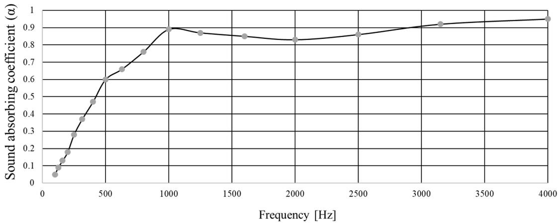
**Fig. 6. Average sound absorption coefficient of the material at the frequencies from 100 to 4000 Hz**
