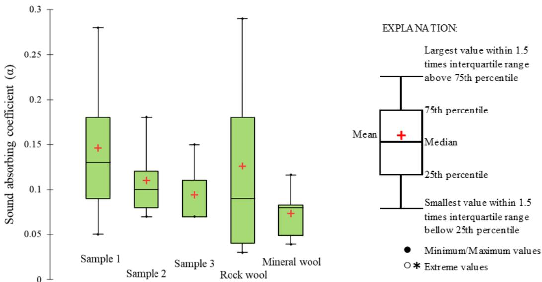
**Fig. 7. Sound absorption coefficients at low frequencies (100-250 Hz)**
