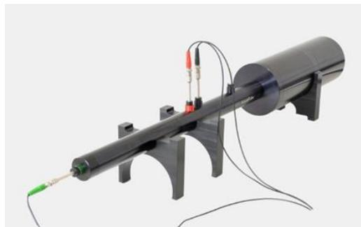
Fig. 5. **AFD 1000 - sound impedance tube [15]**
