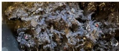
Fig. 3. Shredded textile mixed with a binder
