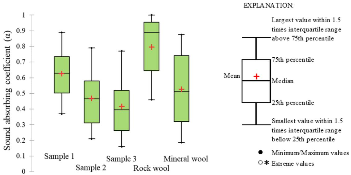
Fig. 8. Sound absorption coefficients at medium frequencies (315-1000 Hz)
