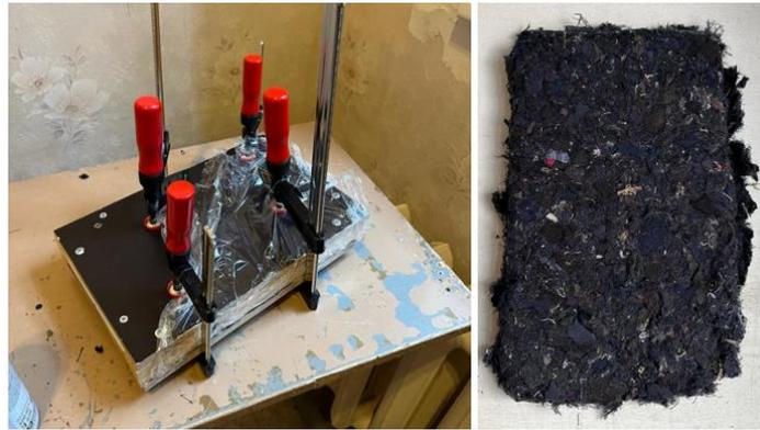
Fig. 4. **Wooden mould with formed material**
