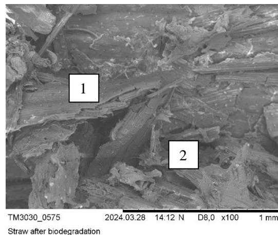
Fig. 2. SEM image – straw with carrageenan after degradation by near-UV radiation ( $\lambda = 405 \text{ nm}$ ): 1 – wheat straw with a damaged surface; 2 – carrageenan damaged and detached, magnification 100x, tabletop microscope HITACHI TM3030
