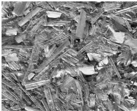
**Fig. 7. Optical microscope image – straw and carrageenan composite before degradation - surface roughness on average 1-1.5 mm, no significant voids between straws, microscope ZEISS Primo Star, grayscale, magnification 20x**
