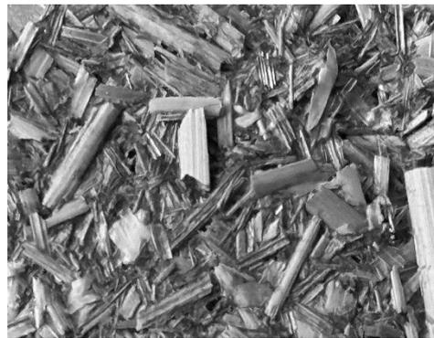
**Fig. 8. Optical microscope image – straw and carrageenan composite after degradation with near-UV radiation ( $\lambda = 405$  nm): – surface roughness on average 2-3 mm, there are significant voids between the straws, microscope ZEISS Primo Star, grayscale, magnification 20x**
