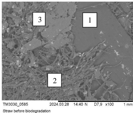
**Fig. 5. SEM image – straw and waste paper glued with carrageenan before degradation:**
