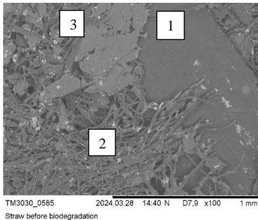
Fig. 5. SEM image – straw and waste paper glued with carrageenan before degradation: 1 – wheat straw; 2 – waste paper; 3 – carrageenan; magnification 100x, tabletop microscope HITACHI TM3030
