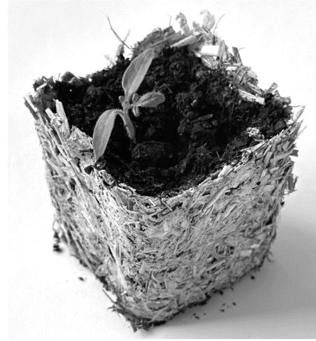
Fig. 4. Finished product – seedling pot. A rough surface of the walls can be observed under the influence of moisture and visible light, the straw-carrageenan composite easily decomposes in contact with the soil
