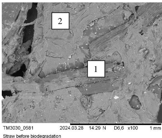
Fig. 1. SEM image – straw glued with carrageenan before degradation: 1 – wheat straw; 2 – carrageenan; magnification 100x, tabletop microscope HITACHI TM3030
