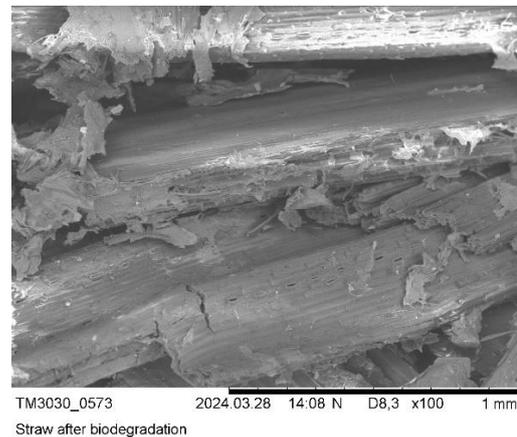
Fig. 6. SEM image – damaged composite of straw, waste paper, and carrageenan after degradation by near-UV radiation ( $\lambda = 405$  nm), magnification 100x, tabletop microscope HITACHI TM3030
