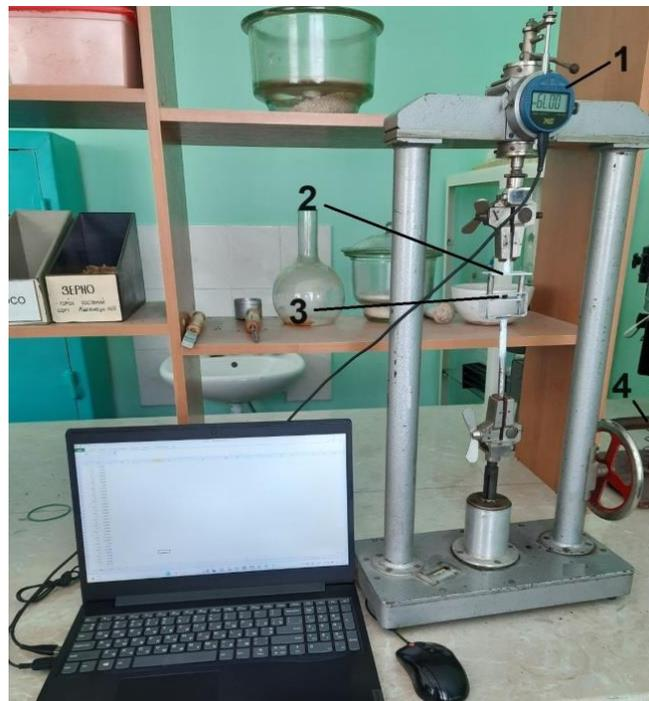
Fig. 3. Picture of the setup for testing the granule strength
