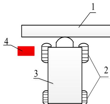
Fig. 2. **Combine harvester with stripper header and grain tray location:** 1 – stripper header; 2 – harvester wheels; 3 – combine harvester; 4 – grain loss measurement tray
