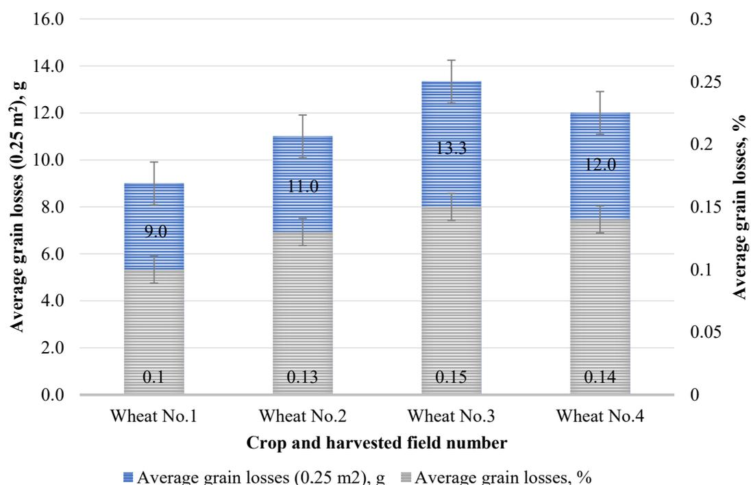
Fig. 3. Wheat grain losses after stripper header
