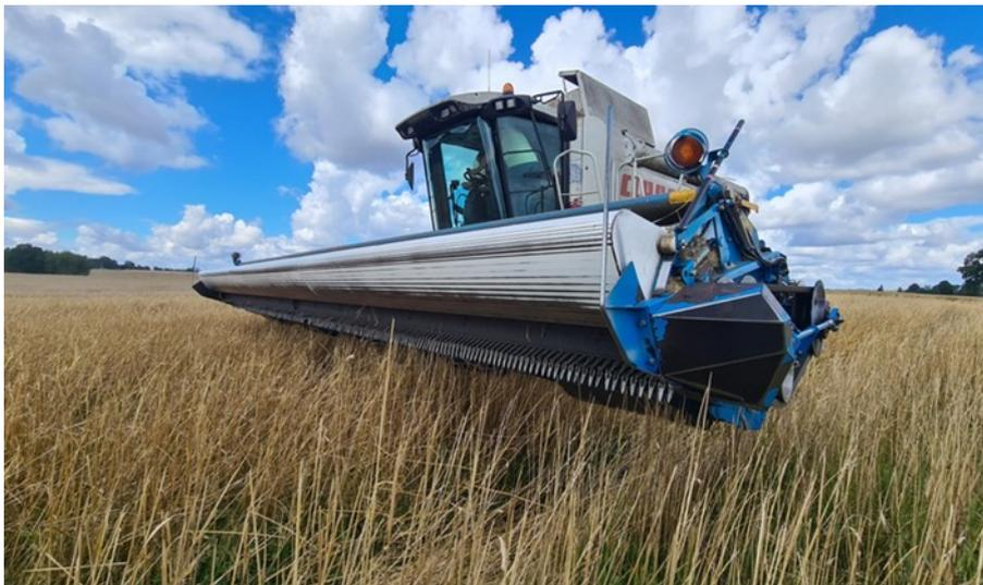
Fig. 1. CLAAS Lexion 550 combine harvester with stripper header
