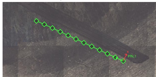
Fig. 11. Hardness measuring tester HM-210D procedure (Sample 280 A)
