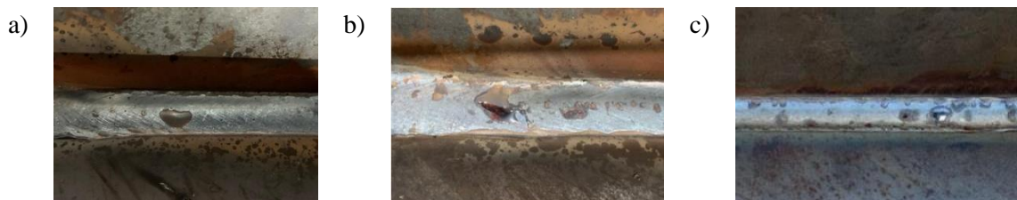
Fig. 5. Amounts of spatters on welding seams with different welding current: a – 280 A; b – 320 A; c – 360 A
