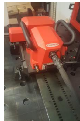
Fig. 2. Welding tractor Fronius® FlexTrack 45 Pro
