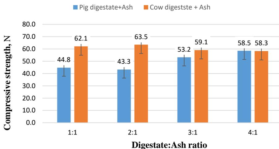
Fig 2. Average breaking force of granules in cross direction in dependence on digestate: ash ratio
