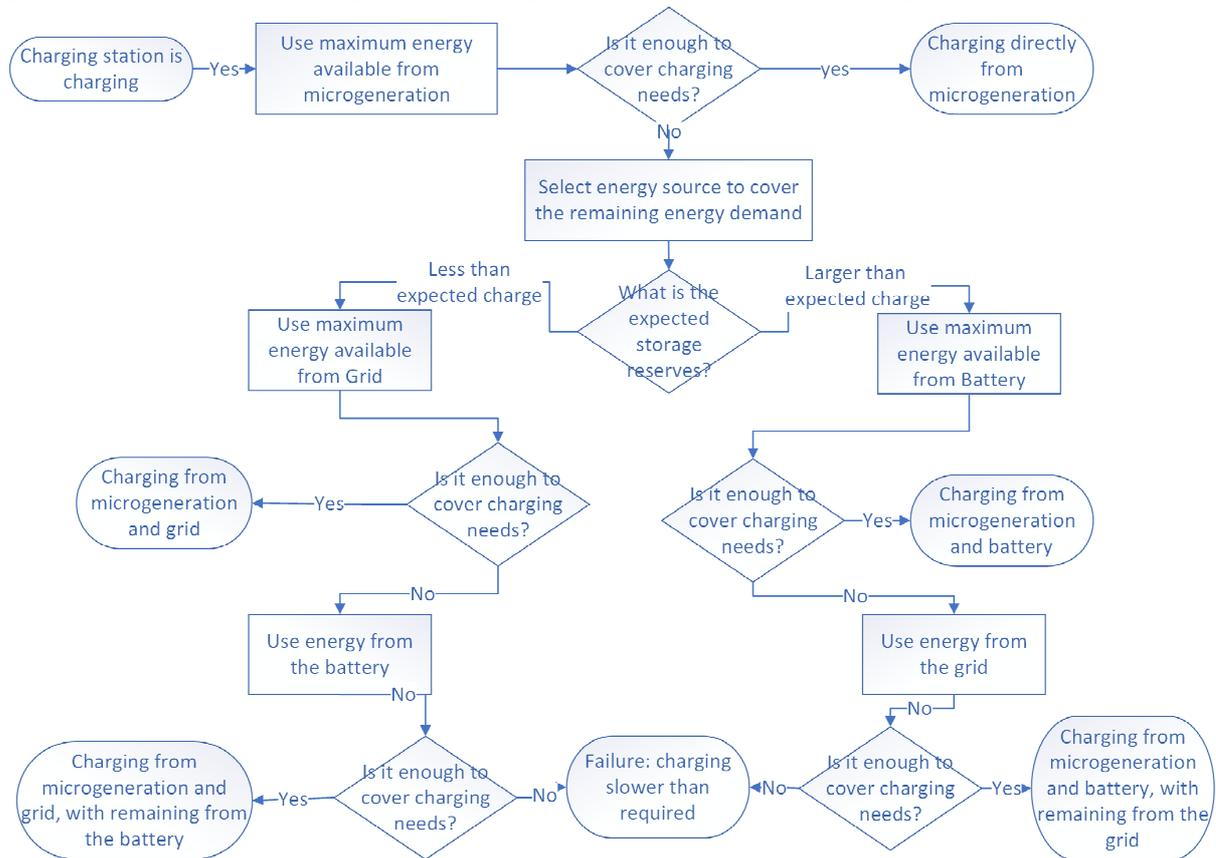
Fig. 3. Energy flow algorithm during charging process
