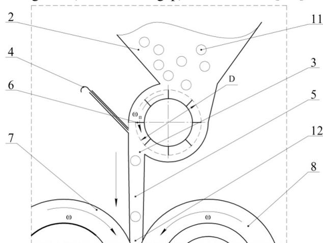
Fig. 1. Scheme of feeding device of PZ-1M forage grain crusher: 1 – frame; 2 – feeding hopper; 3 – window; 4 – flap; 5 – grain feeding channel; 6 – feeding roll ; 7, 8 – rollers for flattening (basic); 9 – electric motor; 10 –vee belt transmission; 11 – grain for flattening; 12 – inter-roll gap
