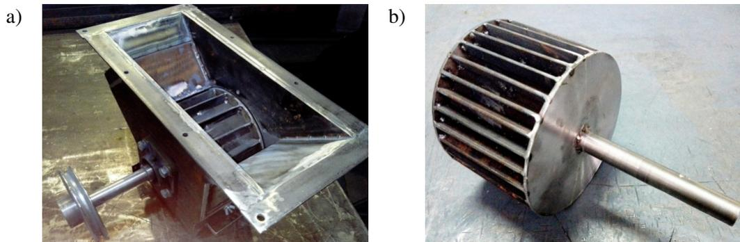
Fig. 2. General view of experimental sample of feeding device (a) and its working tool – feeding roll (b)
