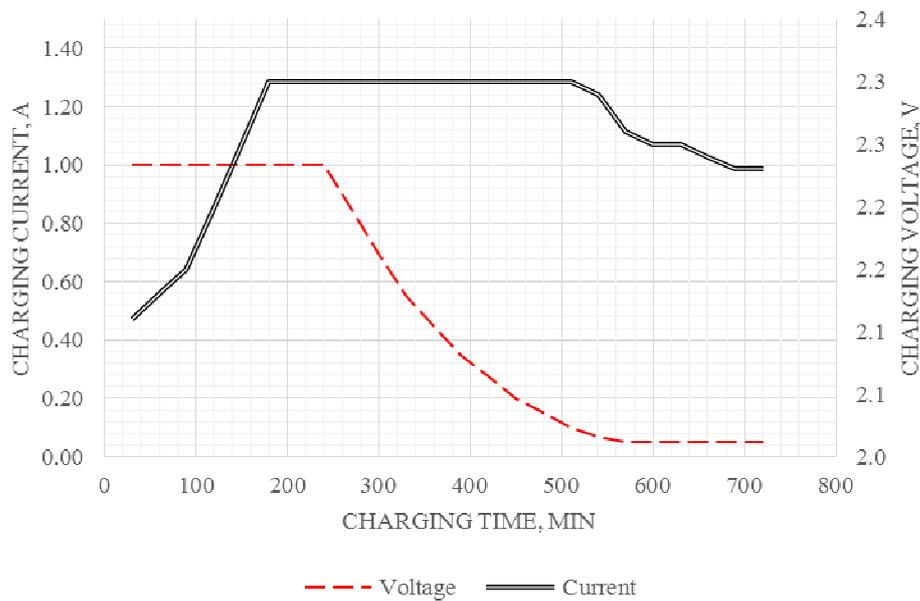
Fig. 3. Experimental results of battery charging voltage and current experiments
