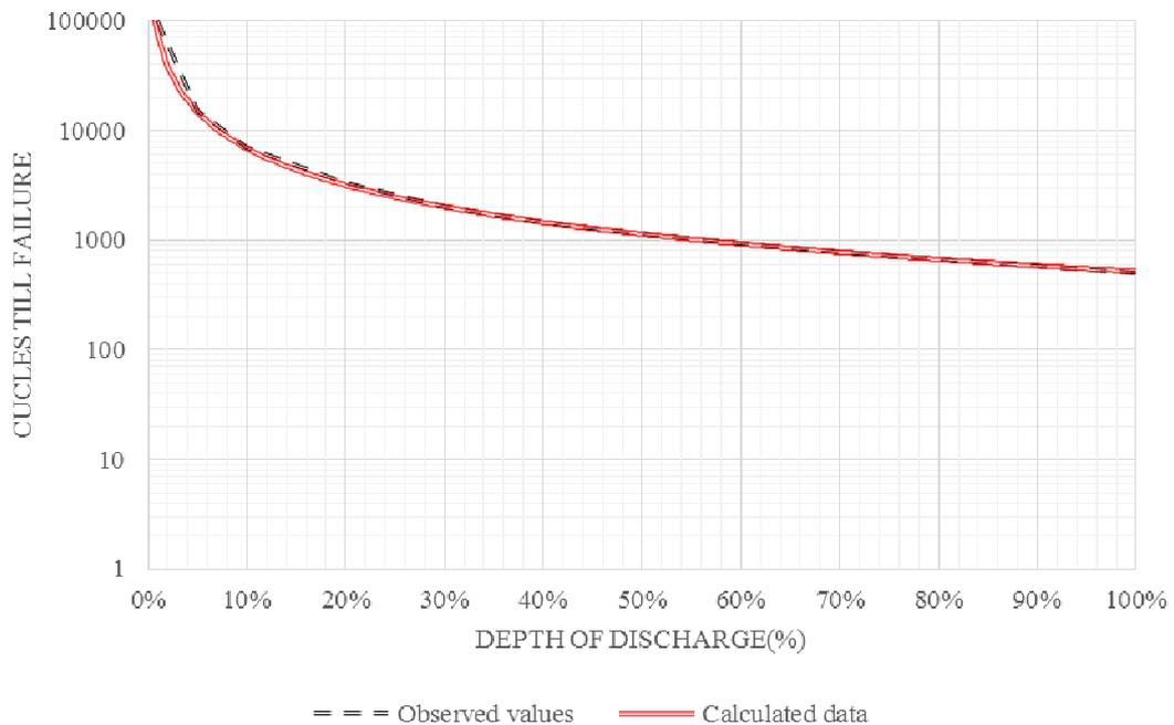
Fig. 7. Cycles till battery failure depending on DoD ( $R^2 = 0.999$ )
