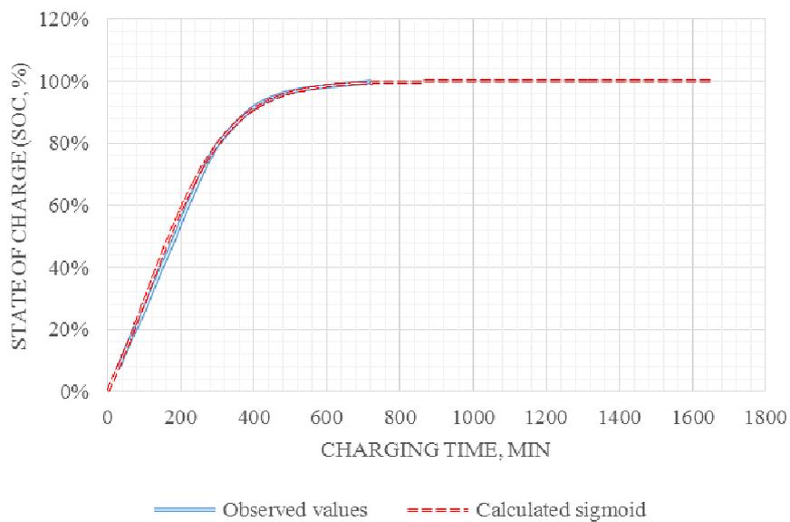
Fig. 4. State of charge depending on charging time
