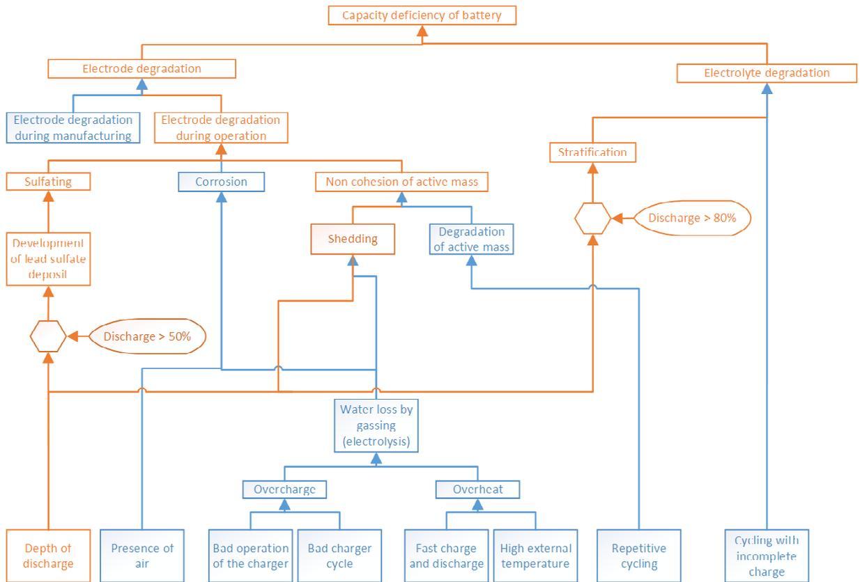
Fig. 6. Causal tree analysis of DoD impact on capacity deficiency of battery
