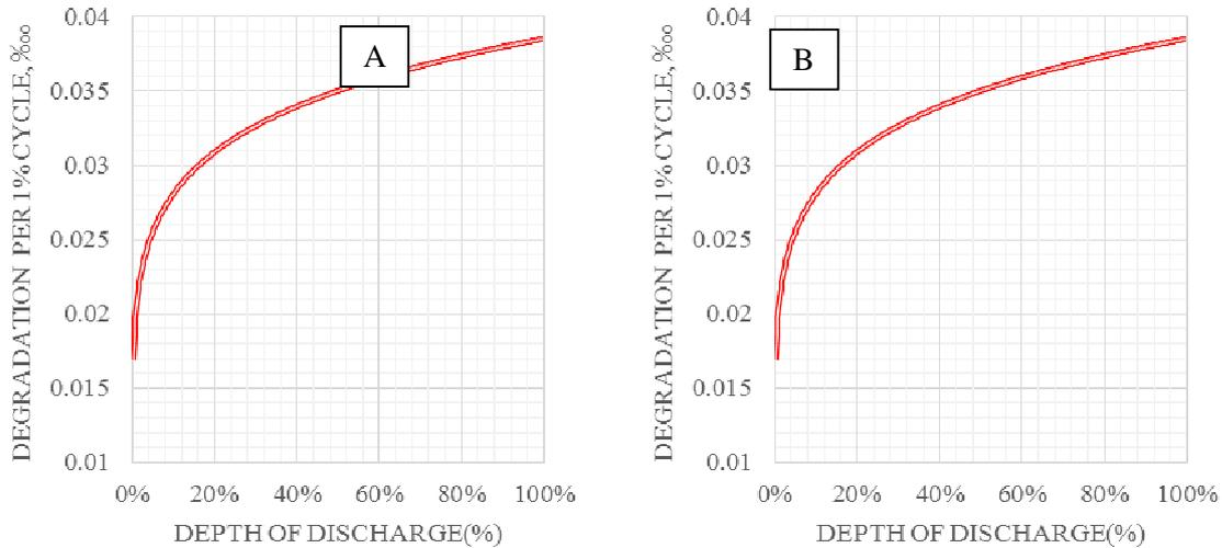
Fig. 8. Degradation of battery capacity: a – basis points per full cycle; b – basis points per 1 % charge cycle
