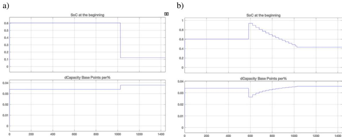
Fig. 5. Capacity loss during charging at ordinary (a) vs wireless (b) charging scenarios (basis point per per cent charged)
