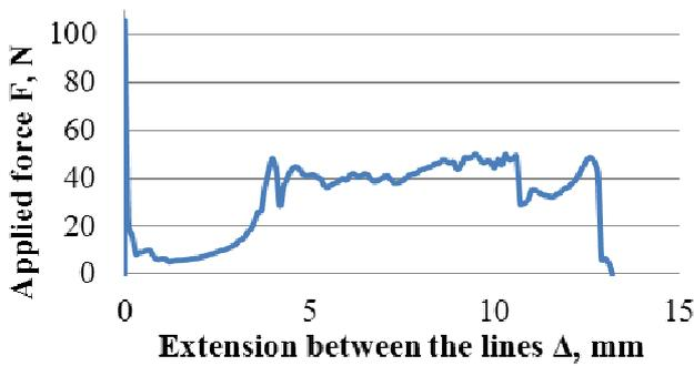
Fig.14. Pull-out of SF at an angle of 10°
