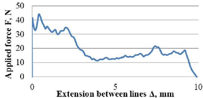
Fig. 5. Pull-out diagram for SF oriented under the angle  $90^\circ$
