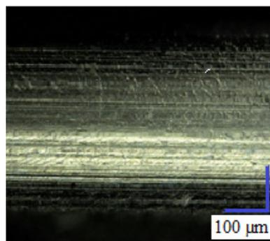
Fig. 2. SF surface before pull-out
