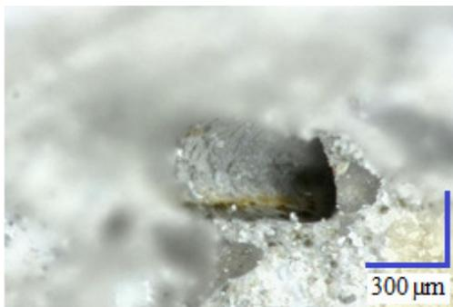
Fig. 6. Surface of channel left by the fibre orientated under  $90^\circ$
