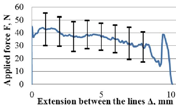
Fig. 19. Average value for samples with fibre angle  $70^\circ$ , where  $F$  – applied force [N] and  $\Delta$  - extension between lines [mm]
