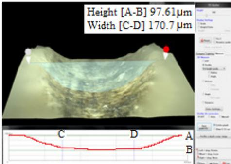
Fig. 4. Surface of the channel left by the fibre
