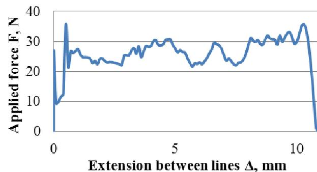
Fig. 7. Pull-out diagram for straight steel fibre orientated at an inclination of  $80^\circ$
