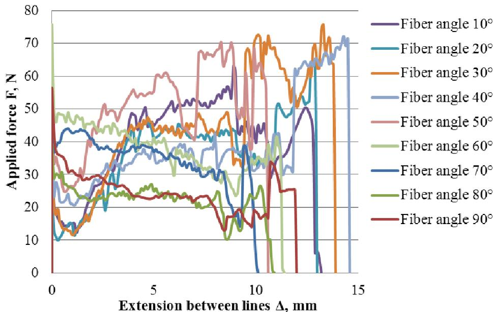
Fig. 21. Average value of pull-out of one SF of the concrete matrix at different inclination angles
