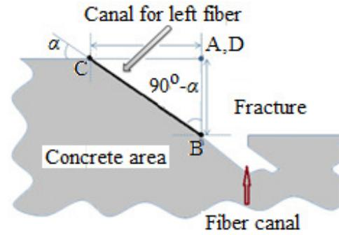
Fig. 10. Canal surface when spalling the concrete and turning the fibre
