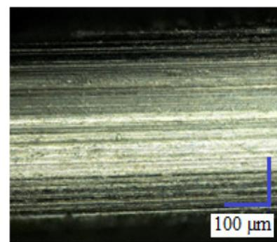
Fig. 3. SF surface after pull-out
