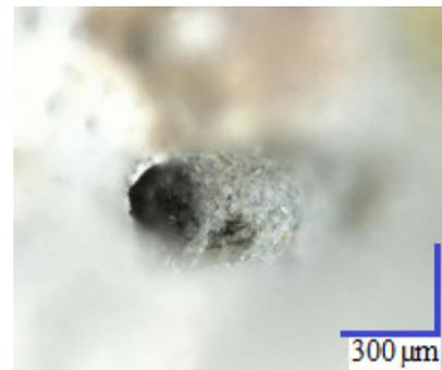
Fig.18. Channel surface left by the oriented fibre at an angle of 10° in sample N55
