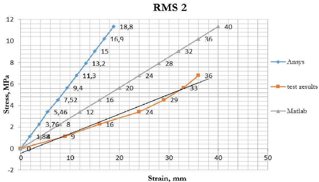
Fig. 8. Stress-strain state of rubber-metal support
