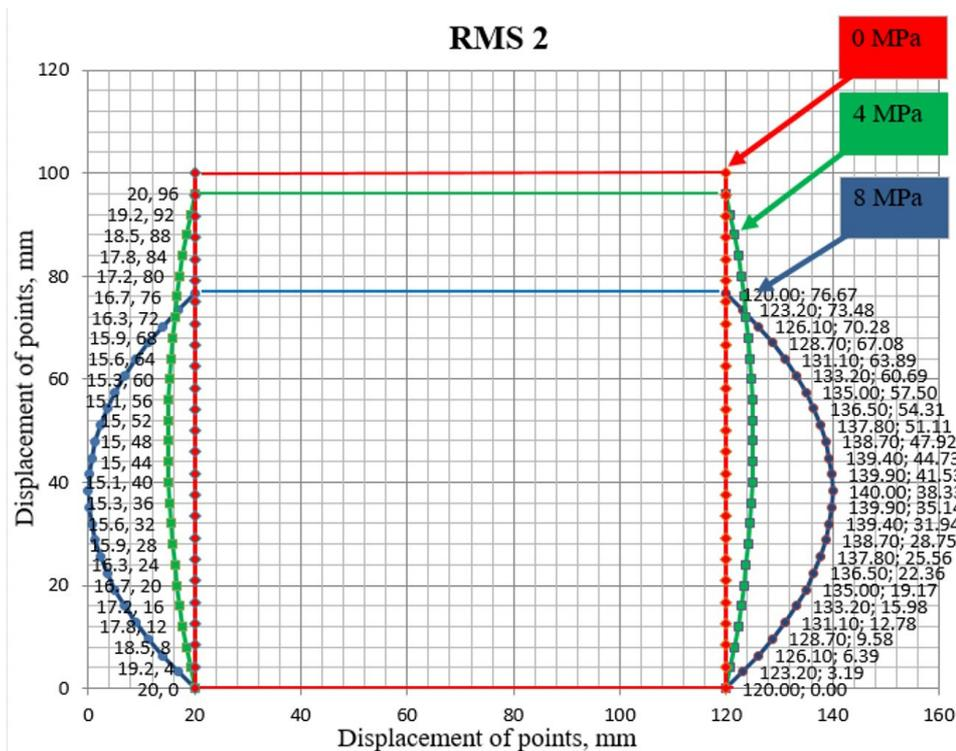
Fig. 4. Displacement of contour points of the researched rubber body of RMS2
