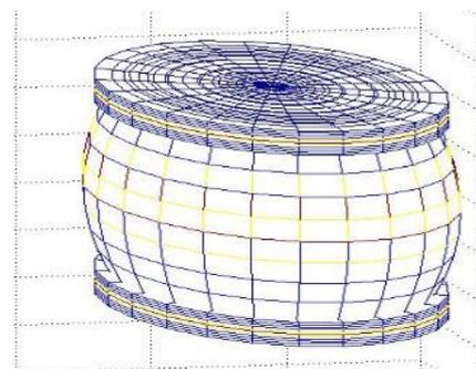
Fig. 3. Compression of rubber-metal supports under a uniformly distributed load
