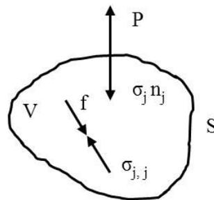
Fig. 1. At any point within the volume  $V$  of the body on the surface  $S$  and the external forces balanced by internal stresses: the stress vector  $\sigma_j$  at the surface with the normal vector  $x_j$
