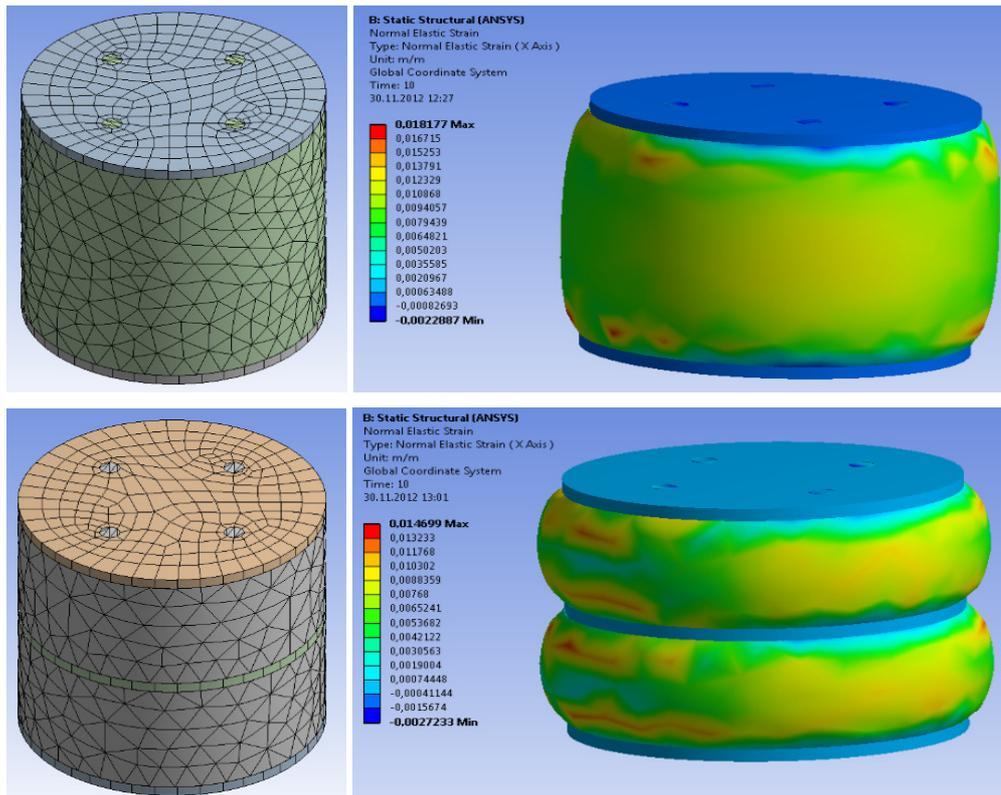
Fig. 7. Modelling of compression RMS2, RMS3 under compression by using the finite element method in ANSYS
