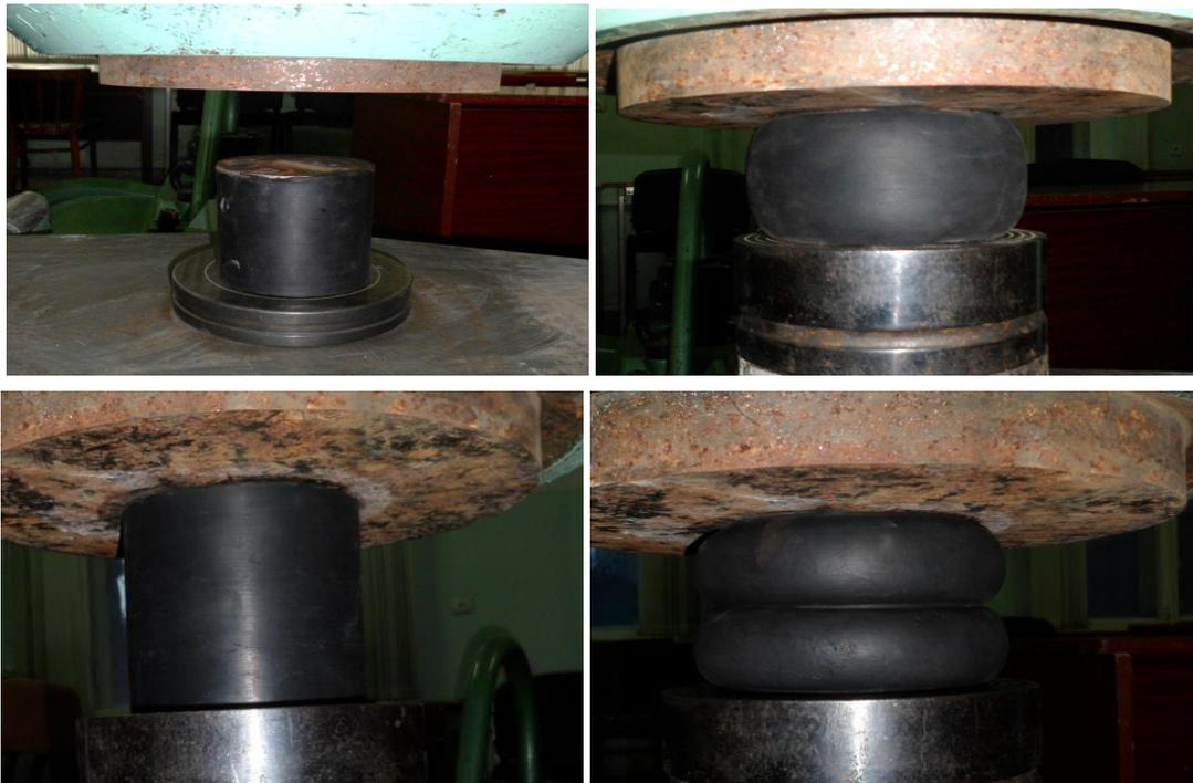
Fig. 6. Compression test of RMS2 and RMS3
