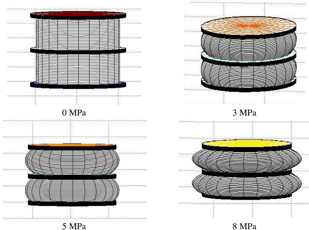
Fig. 5. Process of deformation RMS3 for various compression forces, the distributed load applied to the upper end
