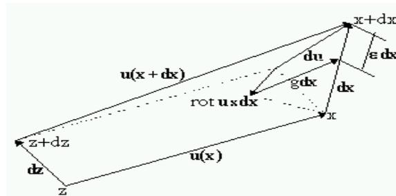
Fig. 2. Decomposition of the vector relative displacement
