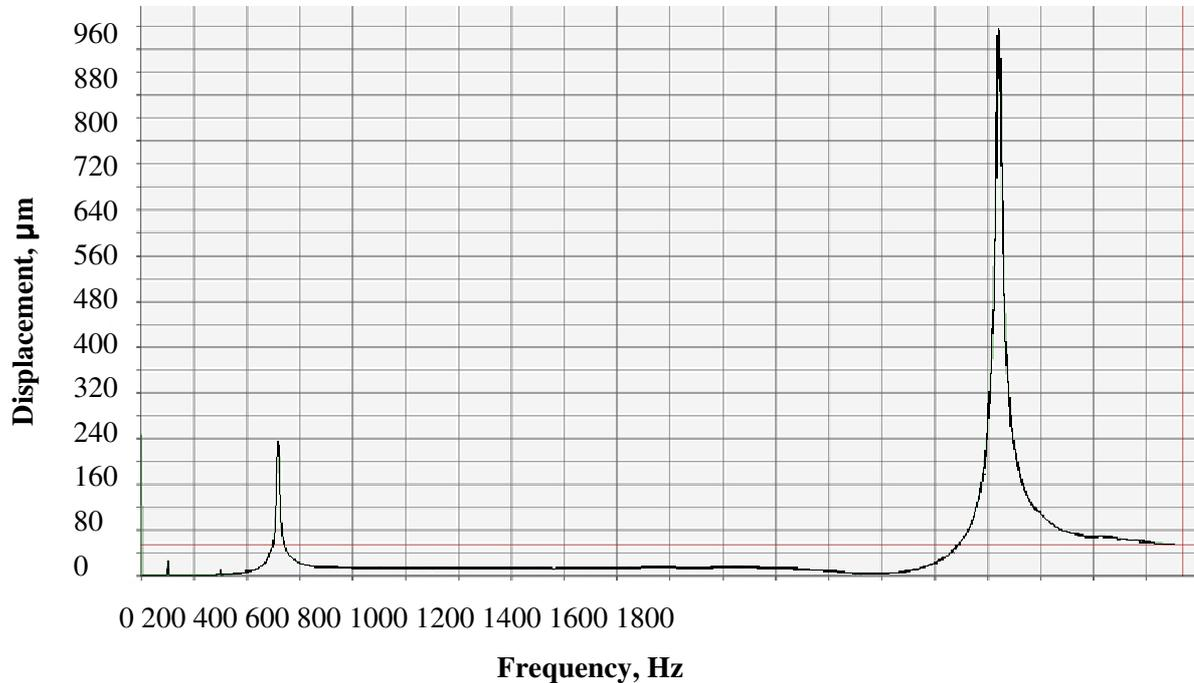
Fig. 3. Frequency response function (FFT) of tool holder
