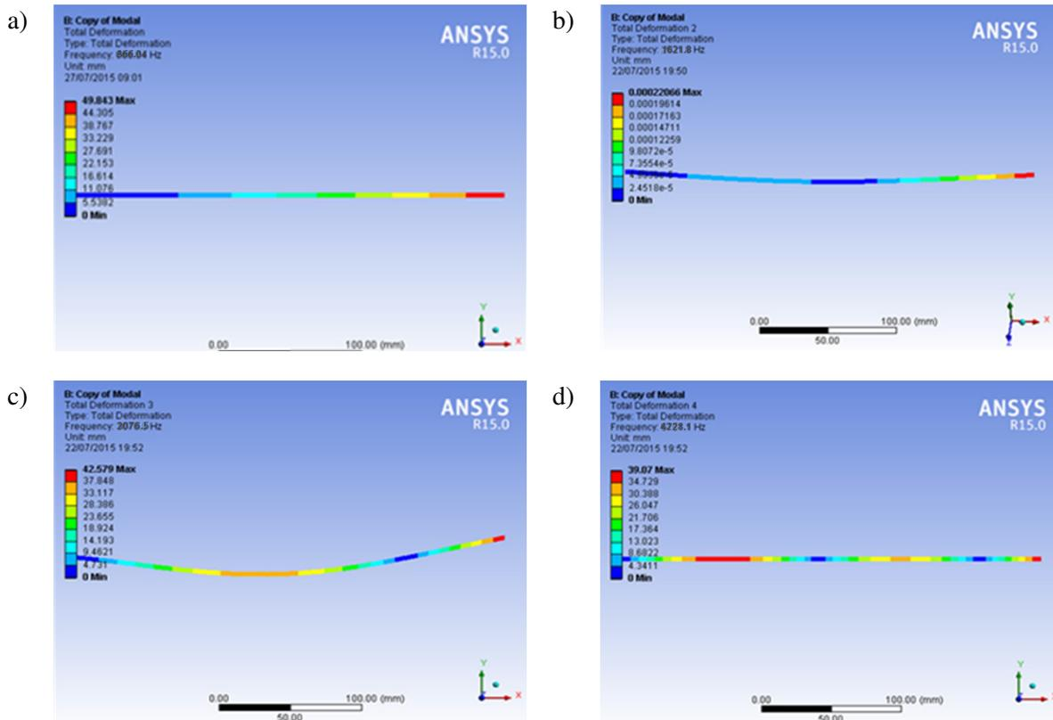
Fig. 2. Mode shapes of tool holder: a – first mode shape; b – second mode shape; c – third mode shape; d – fourth mode shape
