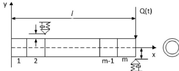
**Fig. 1. Schematic of 2-D finite element model of impacting cantilever**
