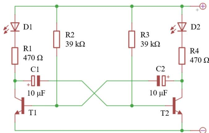
Fig. 1. Scheme of multivibrator
