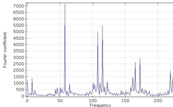
Fig. 6. **Lift force of the moving cylinder in the frequency domain using Fast Fourier Transform in 2DOF case**
