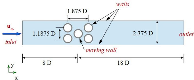
Fig. 2. **Computational domain, dimensions and boundary conditions:**  $D$  is a diameter of the cylinder and  $u_\infty$  is the free-stream velocity
