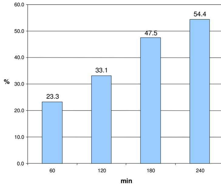
Fig. 4. Mass share of the finest fraction depending on the grinding time
