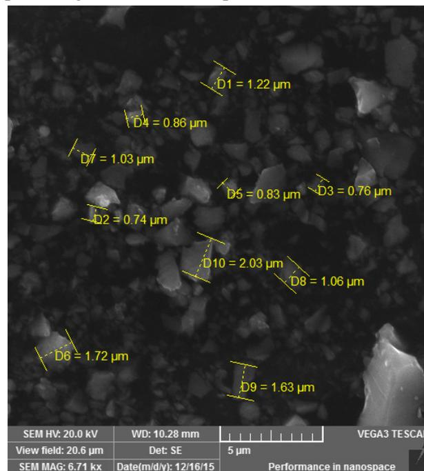
Fig. 4. Detail of the grain fraction  $x < 20$  micron of sample 2
