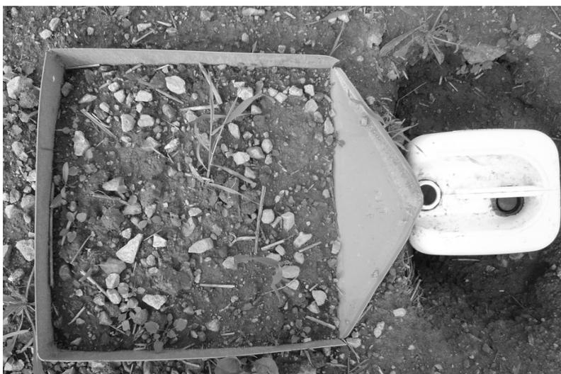
Fig. 1. Drain microplot with drip area 0.16 m<sup>2</sup>
