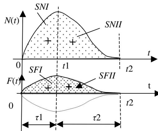
**Fig. 1. Model of collisions in point K:**  $N$  – normal reaction;  $\pm F$  – dry friction force with variable direction ( $\pm$ ) along tangent in contact point  $K$ ,  $\omega_0, \omega_1, \omega_2$  – angular velocity of body in three time moments (initial, in the middle, at the end)
