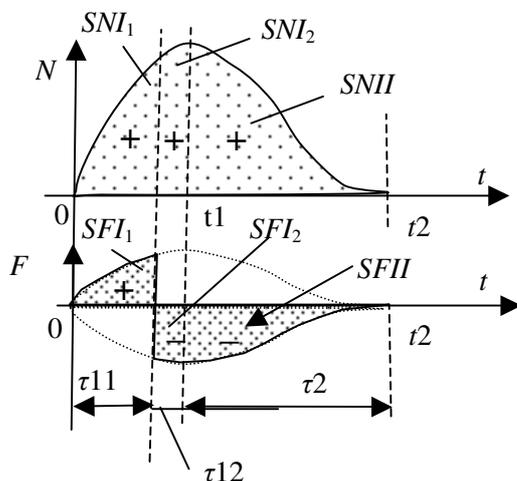
Fig. 3. **Graphic of normal reaction and dry friction force (full slip in two directions) in a case 5:**  $SFI_1$  – dry friction force impulse before reverse in the first phase of impact ( $\tau_{11} \leq \tau_1$ );  $SFI_2$  – negative dry friction force impulse after reverse till  $\tau_1$ ;  $SNI_1, SNI_2$  – parts of normal reaction impulse in the first phase of impact
