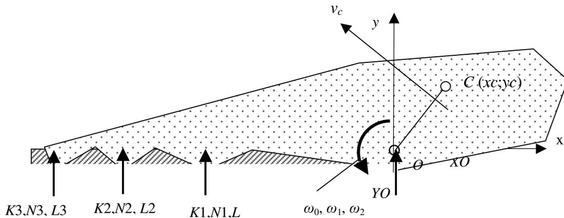
Fig. 7. Model of simultaneous collisions of rotating body in four points
