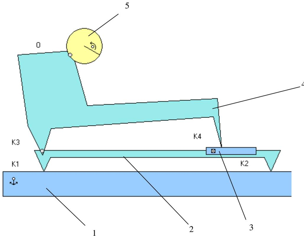
Fig. 8. **Horizontal vibro driver system:** 1 – fundament; 2 – moving platform; 3 – main collision element; 4 – vibro impact actuator; 5 – eccentric, which is driven by electro motor;  $K1$ ;  $K2$ ;  $K3$  and  $K4$  – impacts points;  $O$  – rotation axis of the eccentric
