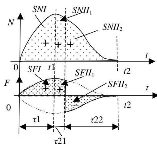
Fig. 4. **Graphic of normal reaction and dry friction force (full slip in two directions) in a case 6:**  $SFI_1$  – dry friction force impulse before reverse in the second phase of impact ( $\tau_1 + \tau_{21} \leq t \leq \tau_1 + \tau_2$ );  $SFII_2$  – negative dry friction force impulse after reverse till  $\tau_1 + \tau_2$ ;  $SNI_1, SNI_2$  – parts of normal reaction impulse in the second phase of impact
