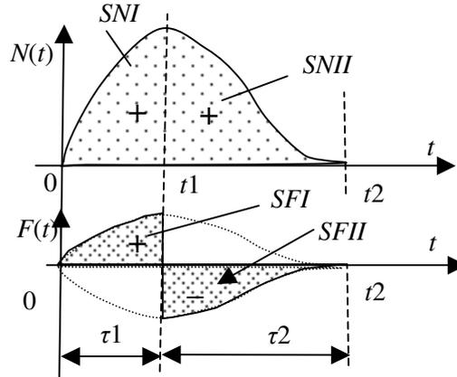
Fig. 6. Diagrams of normal reaction  $N(t)$  and dry friction forces  $F(t)$  in time  $t$  domain
