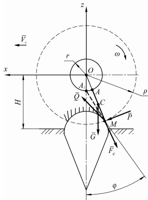
Fig. 1. Equivalent scheme of interaction of the flexible cleaning blade with the beet head
