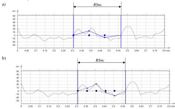
Fig. 3. Representation of flat grinded surface profile in accordance with the number of uncorrelated points along the roughness step *RSm*: a – 3 points; b – 5 points
