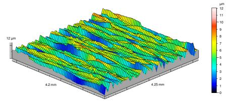
Fig. 4. 3D topography of flat grinded surface
