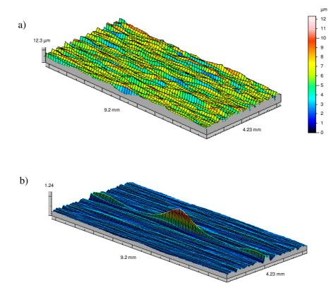
Fig. 1. Flat grinded surface: a – 3D roughness; b – autocorrelation function
