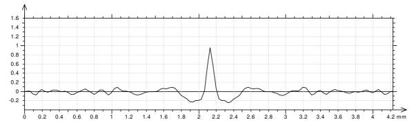
Fig. 2. Autocorrelation function of surface profile
