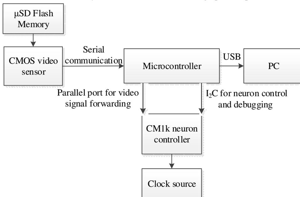
Fig. 2. Sensor structure
