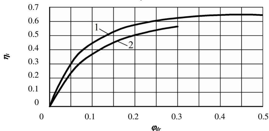
Fig. 1. Dependencies of the draft coefficient of efficiency ( $\eta_t$ ) of a tractor on the utilisation coefficient of the adhesive force ( $\varphi_{dr}$ ), moving across an uncultivated field, after the harvest of cereals (the stubble field) (1) and the field with a soil prepared for sowing (2)
