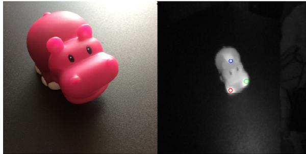
Fig. 6. Identification of markers in captured image from IR camera
