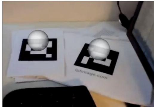
Fig. 2. **Traditional fiducial marker system used in augmented reality**
