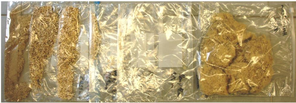
Fig. 2. **Particle size distribution of hemp:** particles retained on the sieve with the largest aperture on the right, with the smallest aperture on the left side; sieves with no captured material (8 and 6.7 mm) were omitted
