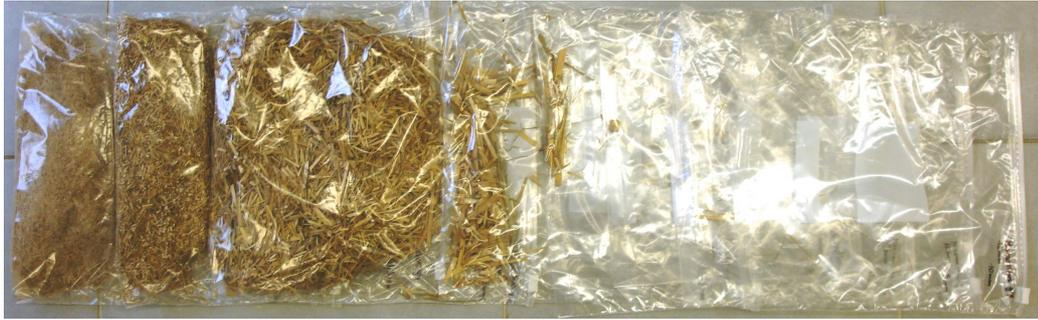
Fig. 4. **Particle size distribution of miscanthus:** particles retained on the sieve with the largest aperture are on the right, with the smallest aperture are on the left side
