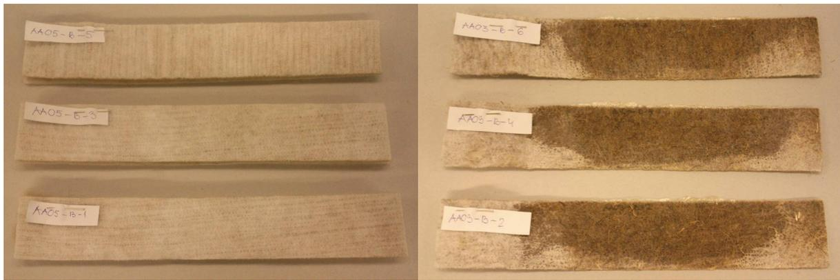
Fig. 2. **NWM and composite sample B strips:** on the left hand side NWM strips AA05-B-1 and AA05-B-3 are cut in the machine direction, strip AA05-B-5 is cut in the cross-machine direction; on the right-hand side composite strips AA05-B-2 and AA05-B-4 are cut in the machine direction, strip AA05-B-6 is cut in cross-machine direction
