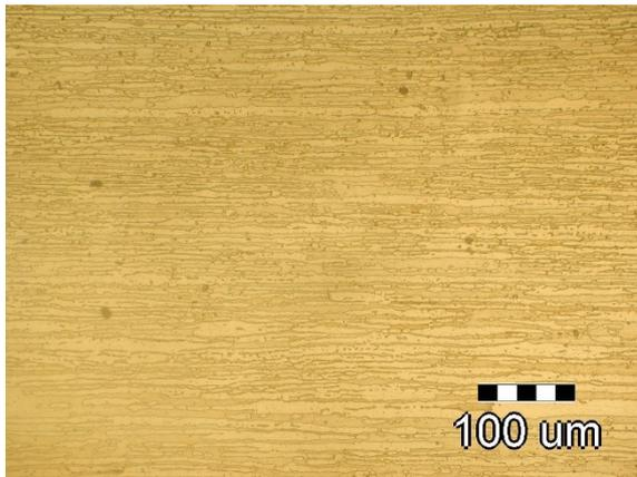
Fig. 1. Microstructure of raw X2CrNiMoSi18-5-3 rolled duplex steel: light etched austenite and dark etched ferrite
