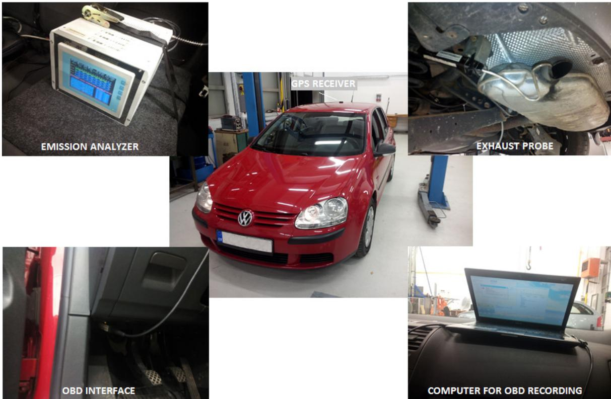
Fig. 1. Equipment of measuring vehicle
