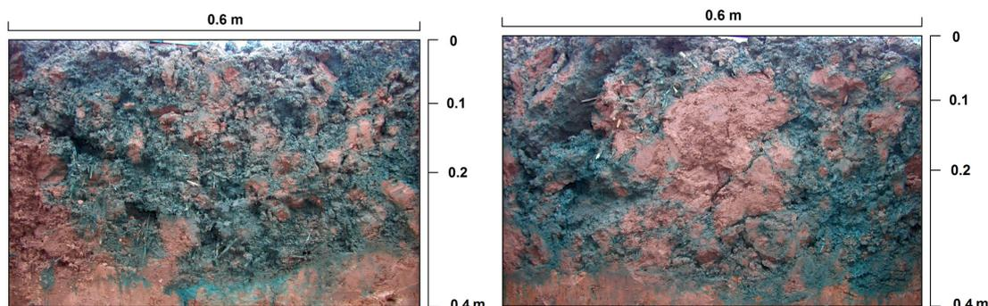
Fig. 5. Simulation of water infiltration into the soil by dye tracer: plough – left, deep cultivator – right
