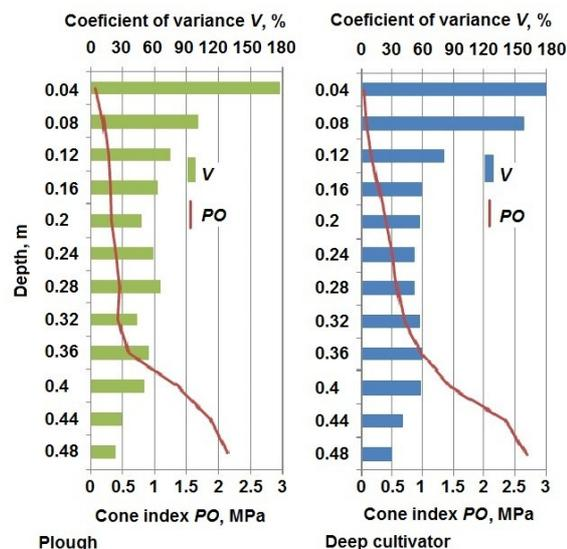
Fig. 4. Average cone index values ( $PO$ , MPa) and coefficient of variation ( $V$ , %) on the surface processed by the deep cultivator and the plough
