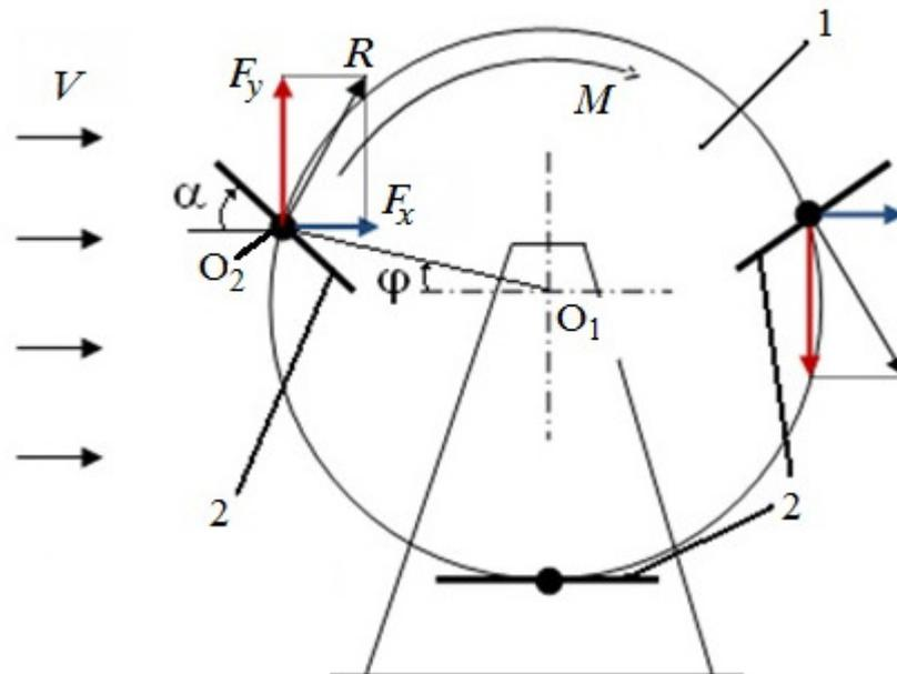
Fig. 1. Principle model of wind device: 1 – rotor; 2 – flat blade
