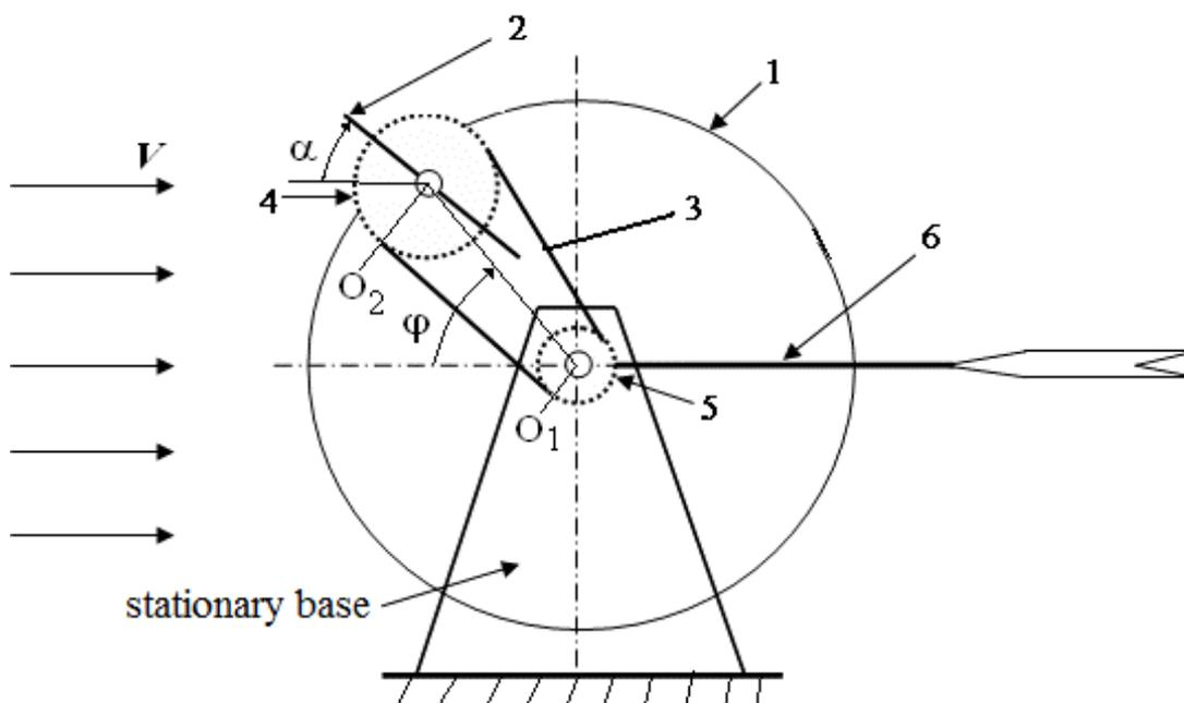
Fig. 8. Kinematic diagram of air flow device: 1 – rotor; 2 – flat blade; 3 – belt transmission; 4 and 5 – pulleys; 6 – tail
