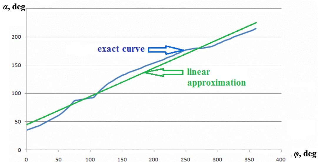
Fig. 7. Linear approximation of relationship between angles  $\varphi$  and  $\alpha$
