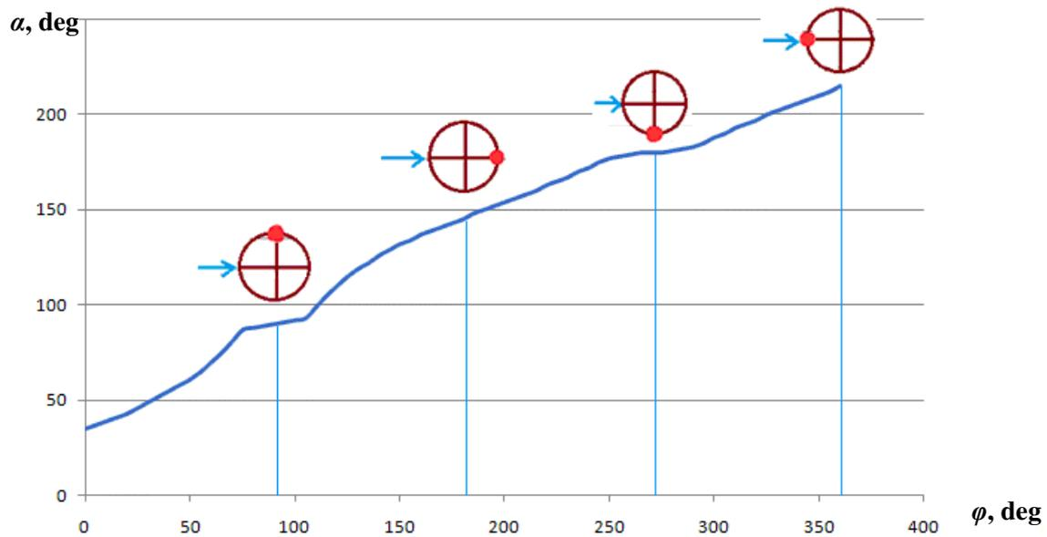
Fig. 6. Relationship between optimal value of blade's angle  $\alpha$  and rotor's turning angle  $\varphi$
