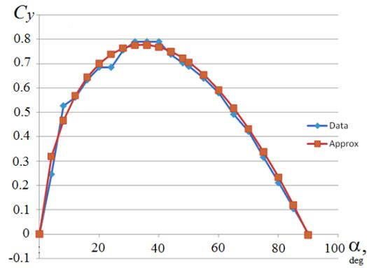
Fig. 4. Lift aerodynamic coefficient  $C_y$  as function of blade's turning angle  $\alpha$
