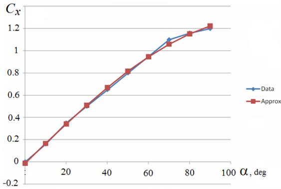
Fig. 3. Drag aerodynamic coefficient  $C_x$  as function of blade's turning angle  $\alpha$
