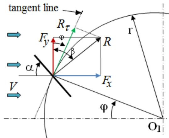
Fig. 5. Decomposition of aerodynamic force  $R$  on components
