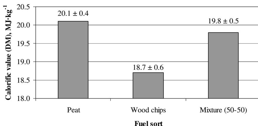
Fig. 3. Calorific value of components and their mixture,  $\text{MJ}\cdot\text{kg}^{-1}$
