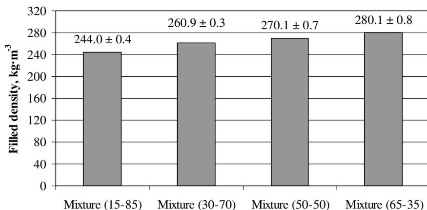
Fig. 2. Filled density of mixtures if peat moisture is 41.7 %; moisture of wood chips is 38.8 %
