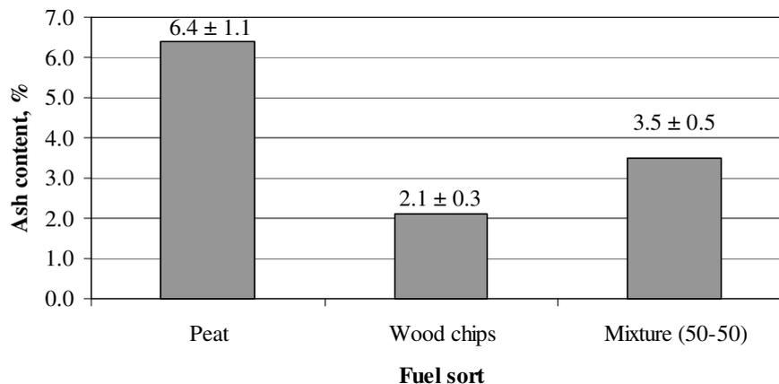
Fig. 4. Ash content of components and their mixture, %
