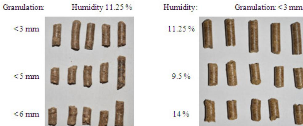
Fig. 4. **Samples of pellets obtained during experiments**
