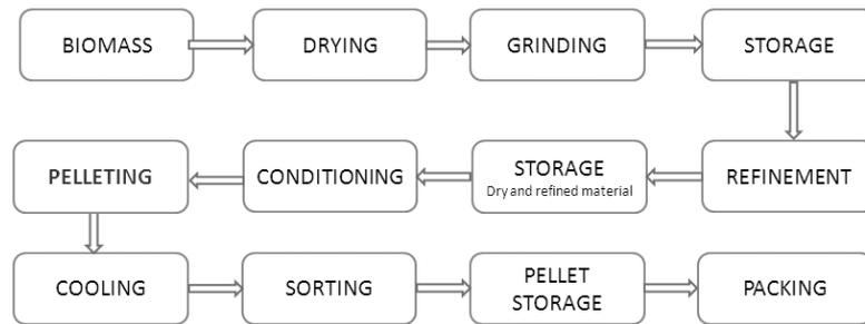
Fig. 1. Process of obtaining pellets from biomass
