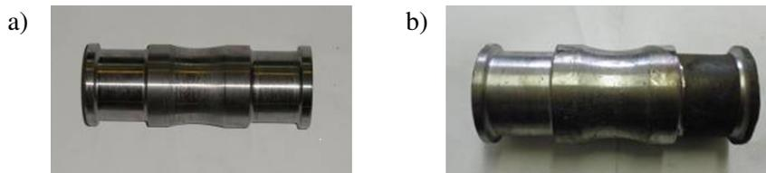
Fig. 4. **Roller:** a – new; b – repaired
