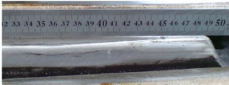
Fig. 3. Longitudinal cracks on frog point after second build-up welding
