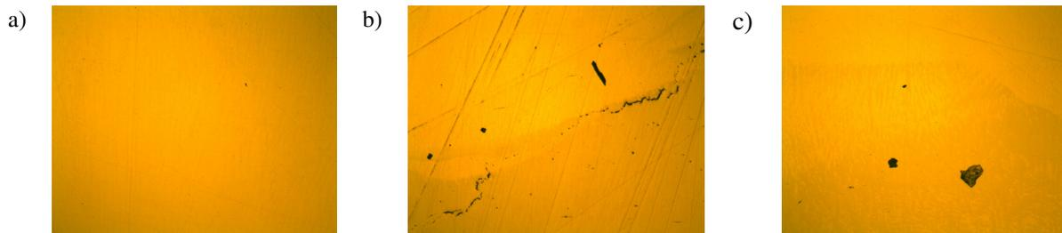
Fig. 7. MMA welded layers (x100): a – good fusion; b – non-fusion; c – inclusions
