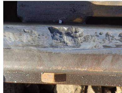
Fig. 6. Spallings in the welded area
