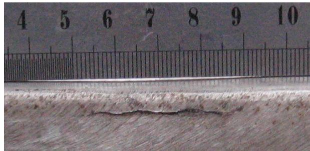
**Fig. 2. Longitudinal crack after first build-up welding**
