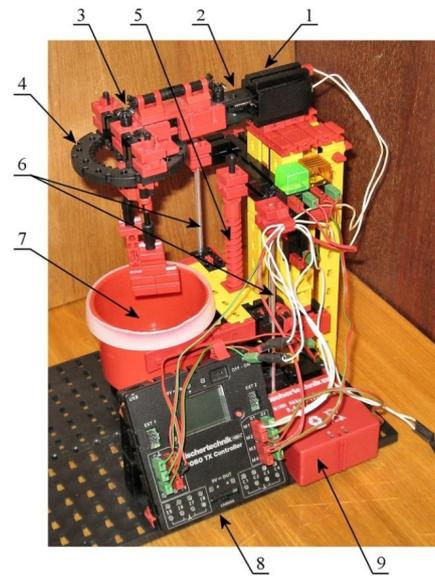
Fig. 5. Industrial mixer mockup from Fischertechnik element: 1 – DC motor; 2 – reduction gear unit; 3 – bevel gearing; 4 – planetary mechanism; 5 – screw gearing; 6 – cylindrical guide; 7 – mixer bowl; 8 – TX controller; 9 – rechargeable accumulator
