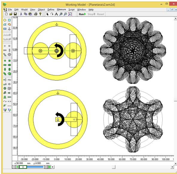
Fig. 4. Planetary mechanism of computer simulation with Working Model
