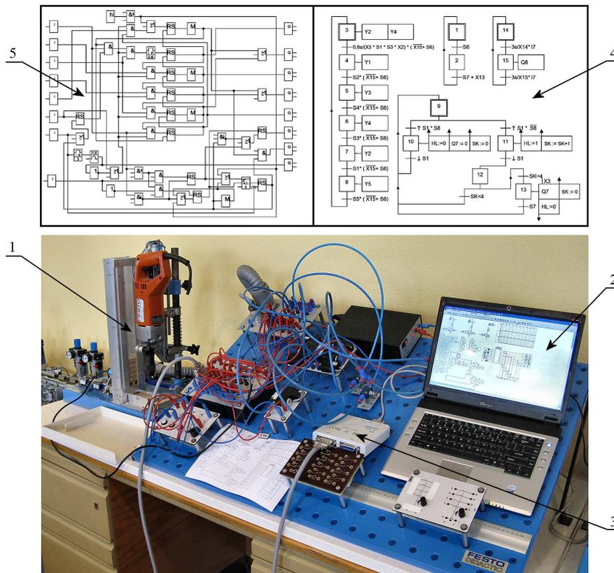
Fig. 1. Festo Didactic learning stand with automatic drilling machine: 1 – drill with preforms magazine; 2 – a computer with FluidSIM software; 3 – EasyPort; 4 – the control algorithm and program Grafcet form; 5 – the control program in the form of FBD
