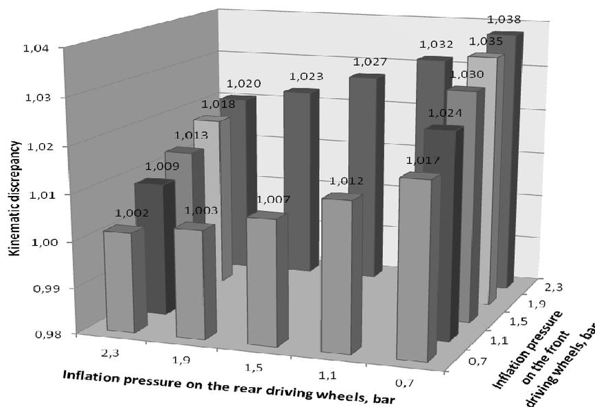
Fig. 2. Kinematic discrepancy of the driving wheels of the tractor driving on different inflation pressure on the front and rear driving wheels
