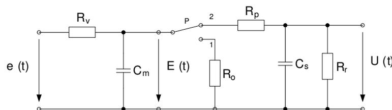
Fig. 6. Model of the thermocouple circuit with the measured object in basic design
