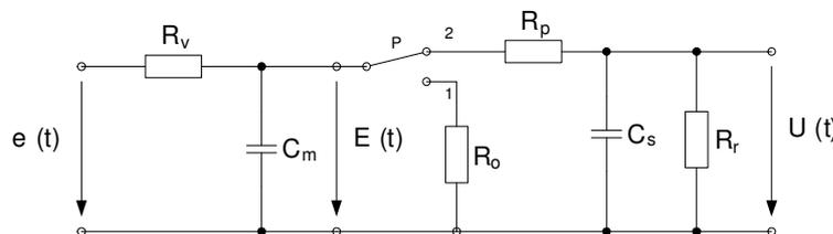
Fig. 1. Model of mutual influence between the thermocouple and the measured object [6]
