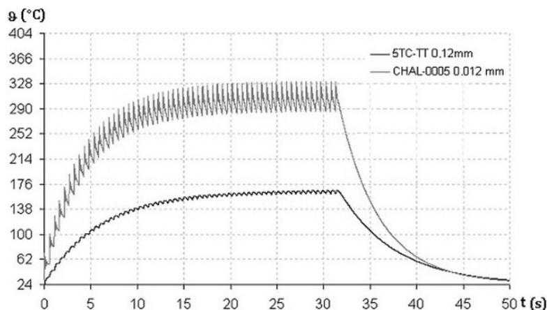
Fig. 9. Model temperature waveform:  $n_p = 60$ ,  $t_1 = 30$  ms,  $t_2 = 500$  ms,  $z = 0.0566$
