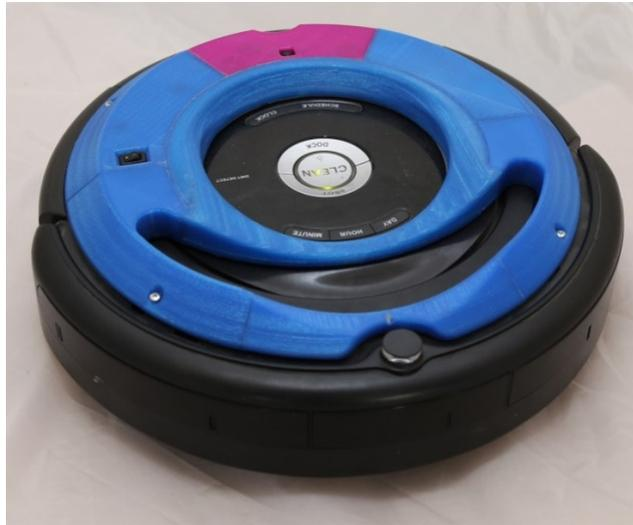
Fig. 7. Roomba 580 with Raspberry Pi add-on
