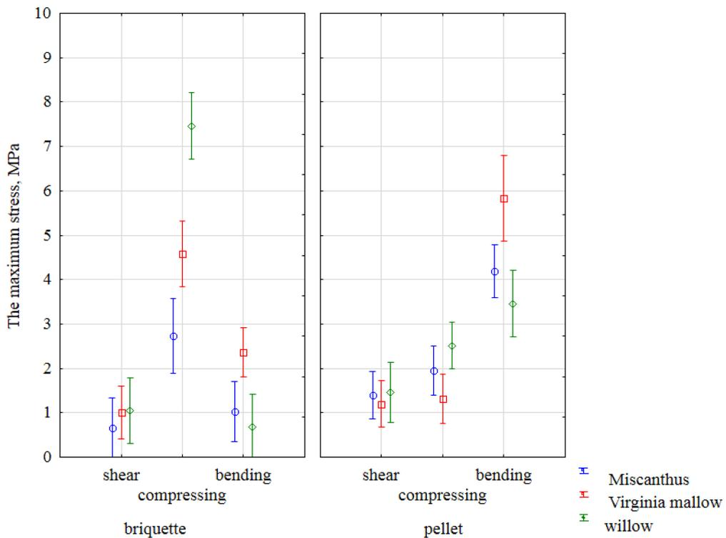
Fig. 2. Interactions between fuel forms, plant species and the load type on the maximum stress of briquettes and pellets
