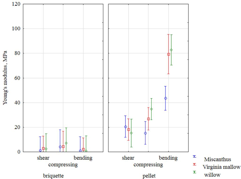
Fig. 1. Interactions between fuel forms, plant species and the load type on the Young's modulus of briquettes and pellets
