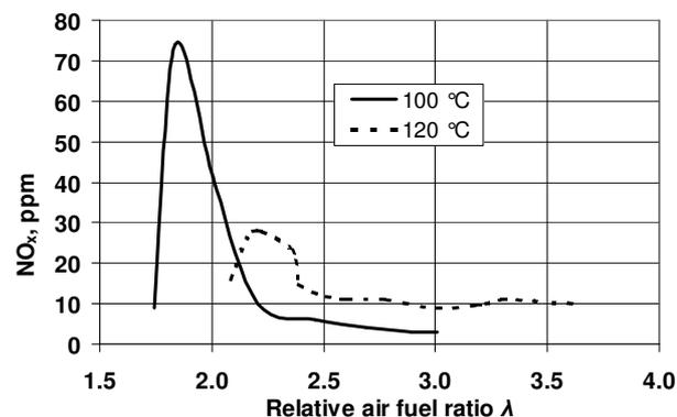
Fig. 7. Dependencies of  $\text{NO}_x$  emitted on air-fuel equivalence ratio and mixture temperature
