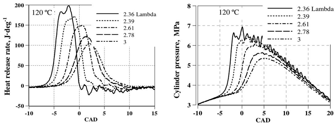
Fig. 4. Influence of equivalence air-bioethanol ratio on the heat release ratio and cylinder pressure
