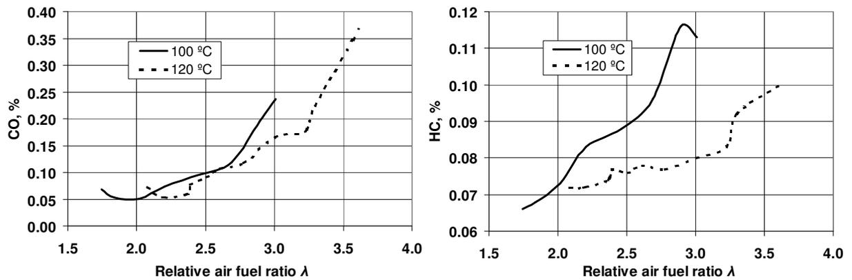
Fig. 8. Dependencies of CO and HC emitted on air-fuel equivalence ratio and mixture temperature
