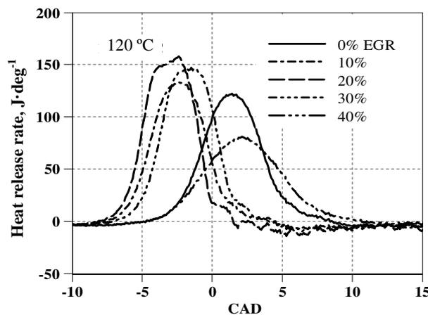
Fig. 5. Influence of EGR on the heat release rate
