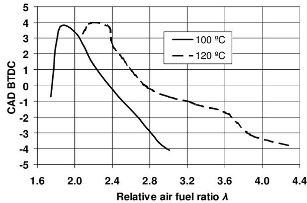
Fig. 1. Dependencies of bioethanol auto ignition with regard to TDC on air-fuel equivalence ratio and mixture temperature
