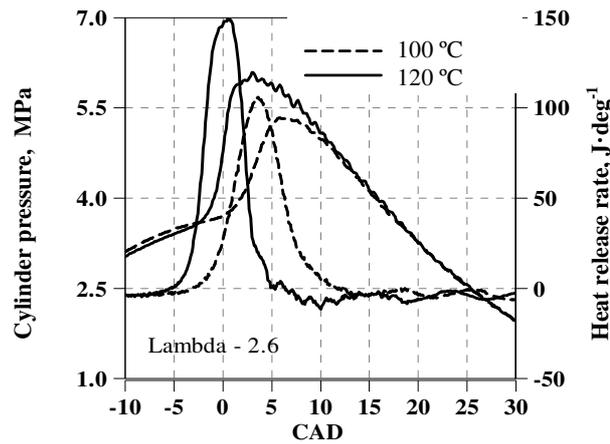
Fig. 3. Dependencies of the heat release rates and cylinder pressure with regard to TDC on mixture temperature
