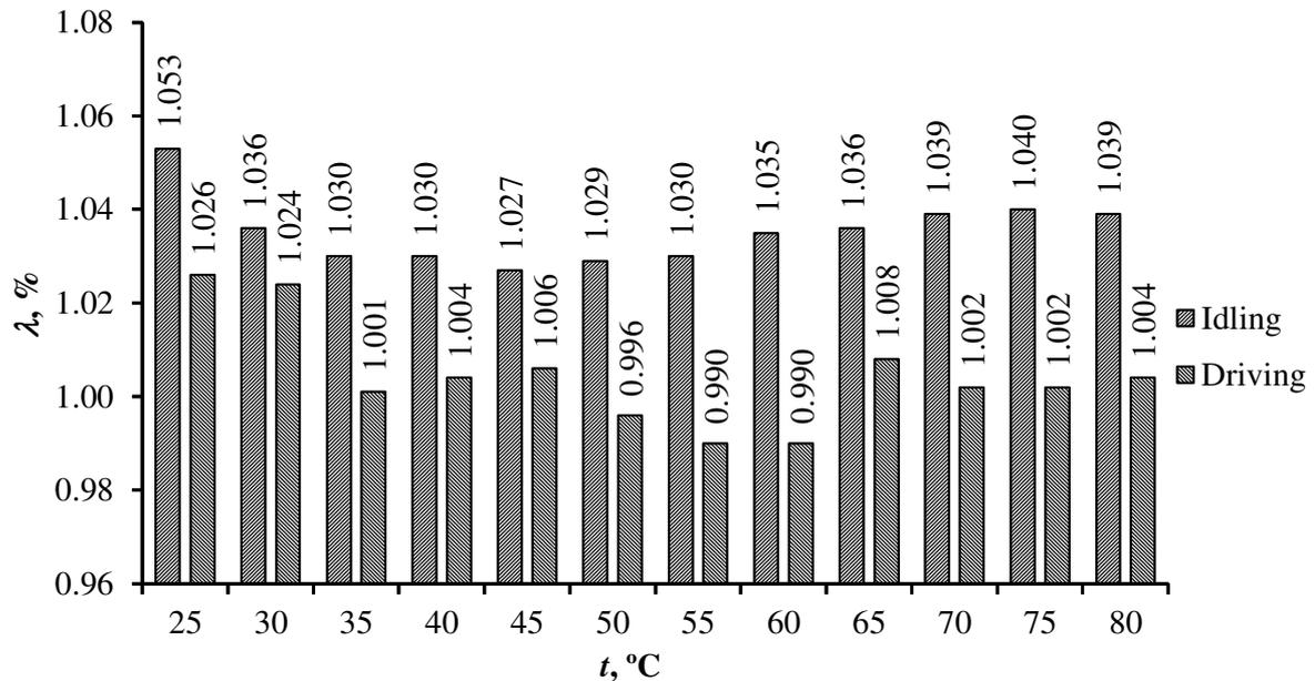
Fig 6.  $\lambda$  changes in exhaust gases
