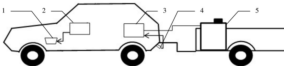
Fig. 1. **Interconnection scheme of the automobile and measuring equipment:** 1 – OBD; 2 – computer; 3 – analyser; 4 – exhaust gases; 5 – generator
