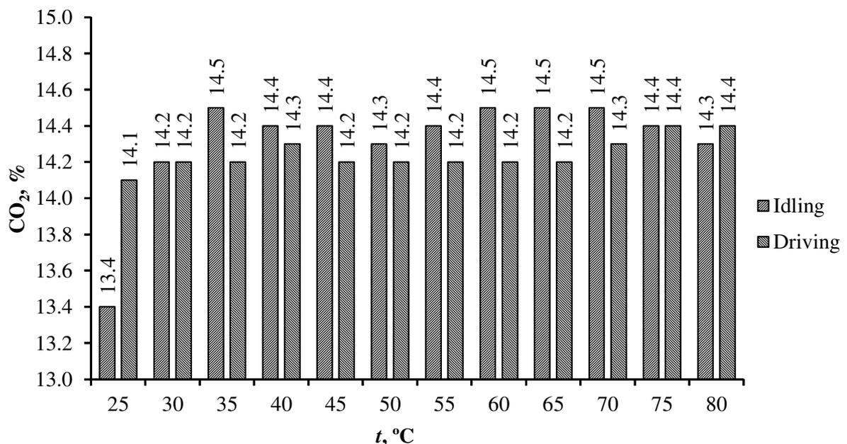
Fig. 3. Changes of the amount of CO<sub>2</sub> in exhaust gases
