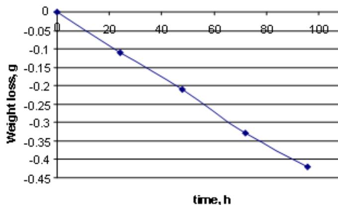
Fig. 5. Weight losses of the zinc galvanised samples exposed to a 5 % acetic acid anhydride solution
