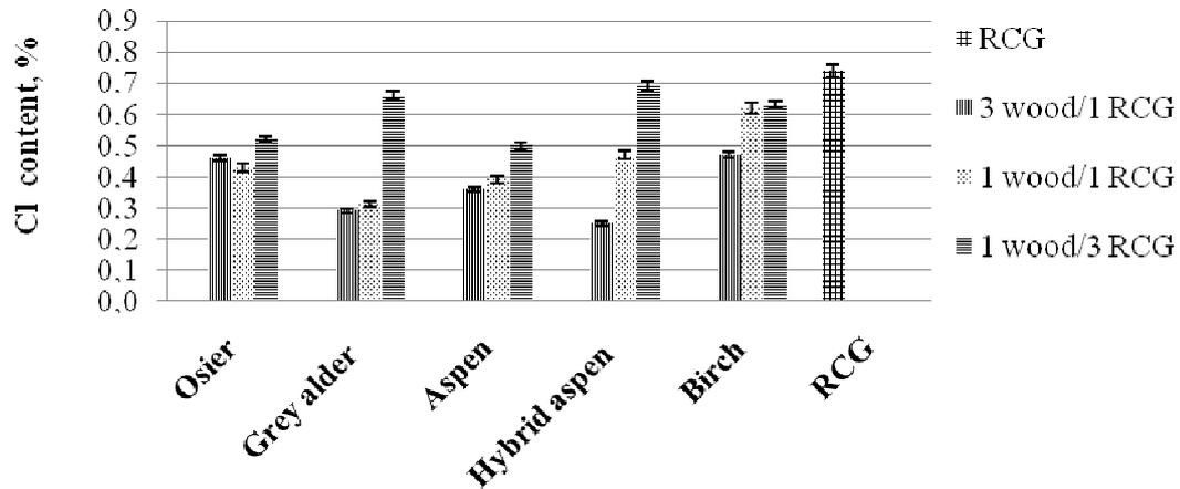
Fig. 2. Chlorine content in reed canary grass and timber pellets
