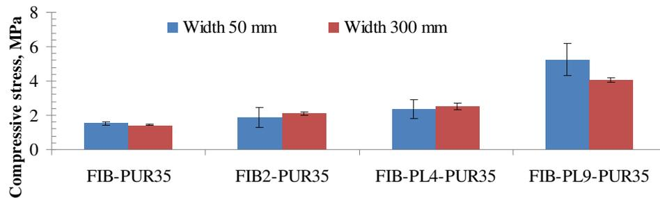
Fig. 3. Compressive stress assessment of test specimens with different widths (50 and 300 mm)
