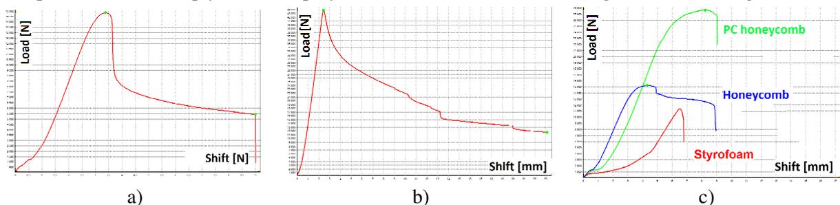
Fig. 4. Stress diagrams during compressive test (buckling resistance)
