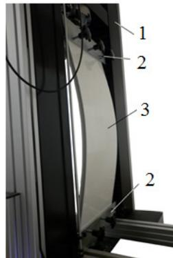
Fig. 1. **Testing equipment:** 1 – testing machine; 2 – fixing apparatus; 3 – specimen
