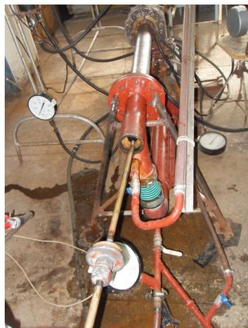
Fig. 6. Charging of seed batch in active zone of experimental vortex cavitator
