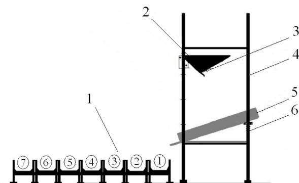
Fig. 1. Schematic view of the stationary experimental stand used for seed sorting based on their rigidity: 1 – troughs designed for sorted seed fractions; 2 – seed feed hopper; 3 – adjustable valve; 4 – frame; 5 – inclined plane; 6 – inclination adjustment mechanism
