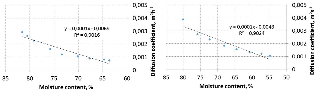
Fig. 5. The diffusion coefficient  $D(c)$  depending on the moisture concentration at different drying temperatures with 20 mm thickness: a – 65 °C; b – 85 °C
