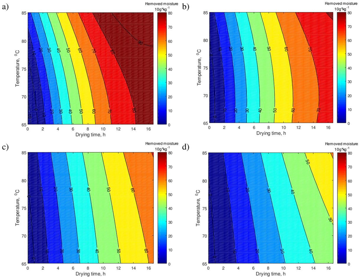
Fig. 2. The average removed moisture changes in potato samples dependence from drying temperature and drying time at different thickness: a – 5 mm; b – 10 mm; c – 15 mm; d – 20 mm
