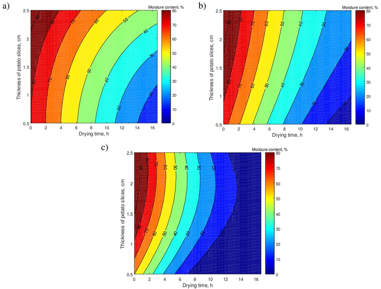
Fig. 3. The average moisture content changes in potato samples with different thickness during drying with different temperatures: a – 65 °C; b – 75 °C; c – 85 °C
