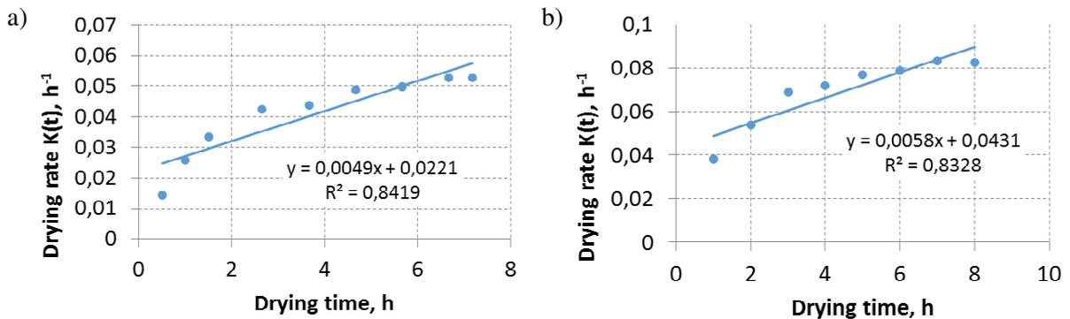
Fig. 4. The drying coefficient depending on the moisture concentration at different drying temperatures with 20 mm thickness: a – 65 °C; b – 85 °C
