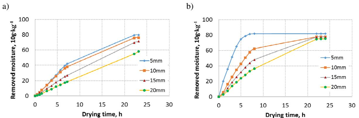
**Fig. 1. The removal moisture content changes in potato samples depending from drying time and sample thickness at temperatures: a – 65 °C; b – 85 °C**
