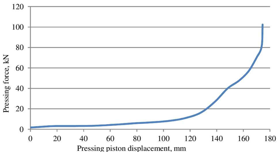
Fig. 2. **Pressing mechanism force – displacement curve**
