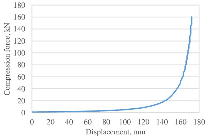
Fig. 4. Compression force characteristic for spring element
