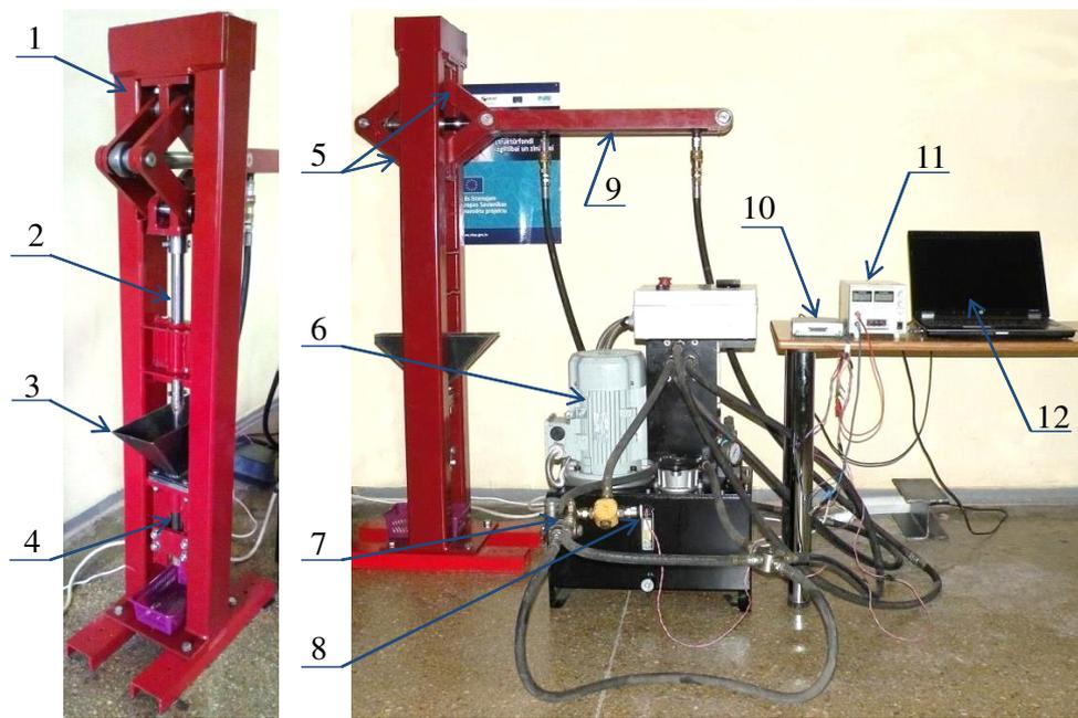
Fig. 1. **Experimental briquetter:** 1 – frame; 2 – pressing piston; 3 – container; 4 – tapered pressing die; 5 – rhombus linkage mechanism; 6 – engine; 7 – flow control valve; 8 – pressure sensor; 9 – drive cylinder; 10 – Data Logger Pico; 11 – power supply; 12 – computer
