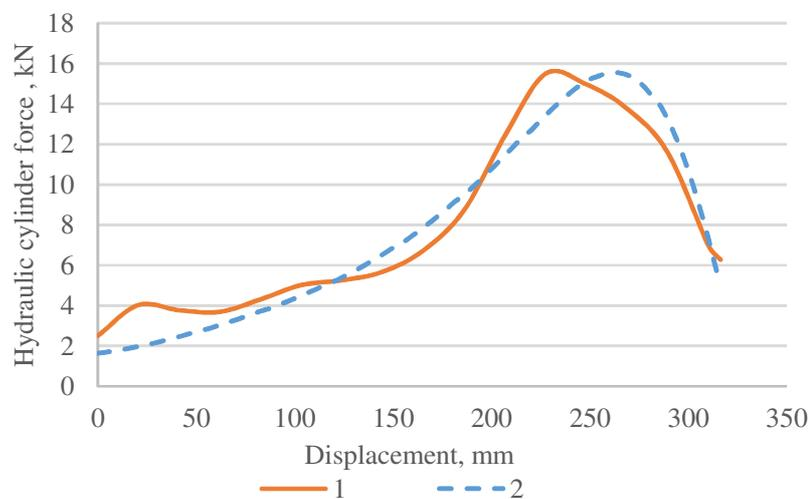
Fig. 5. Hydraulic cylinder force – displacement characteristic
