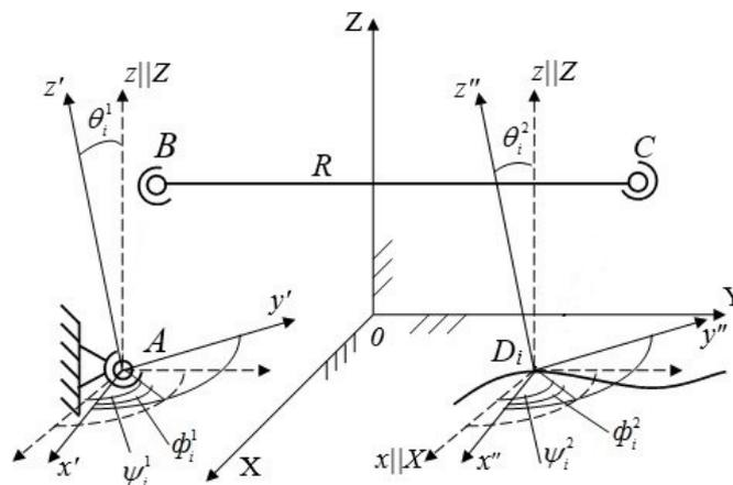
**Fig. 1. Equivalent four-link initial kinematic chain ABCD**
