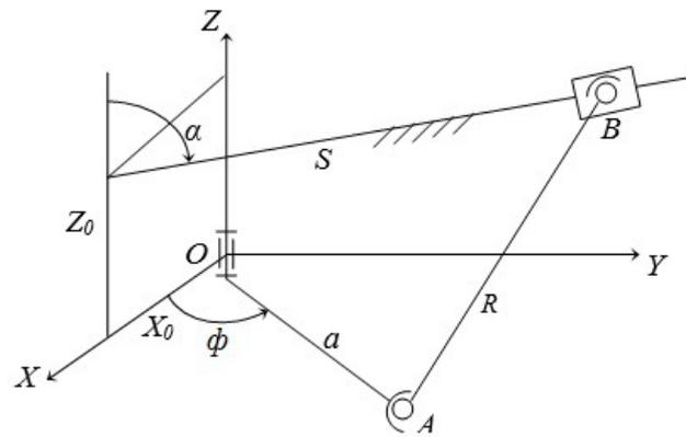
Fig. 5. Equivalent four-link initial kinematic chain *OAB*
