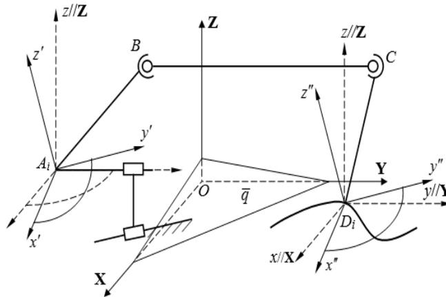
Fig. 2. Equivalent four-link initial kinematic chain ABCD
