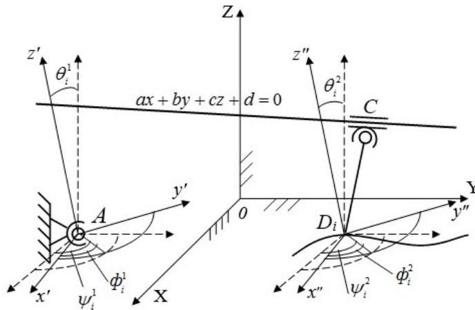
Fig. 3. Equivalent four-link initial kinematic chain ACD
