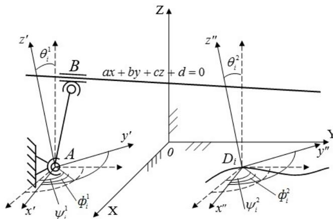
Fig. 4. Equivalent four-link initial kinematic chain ABD
