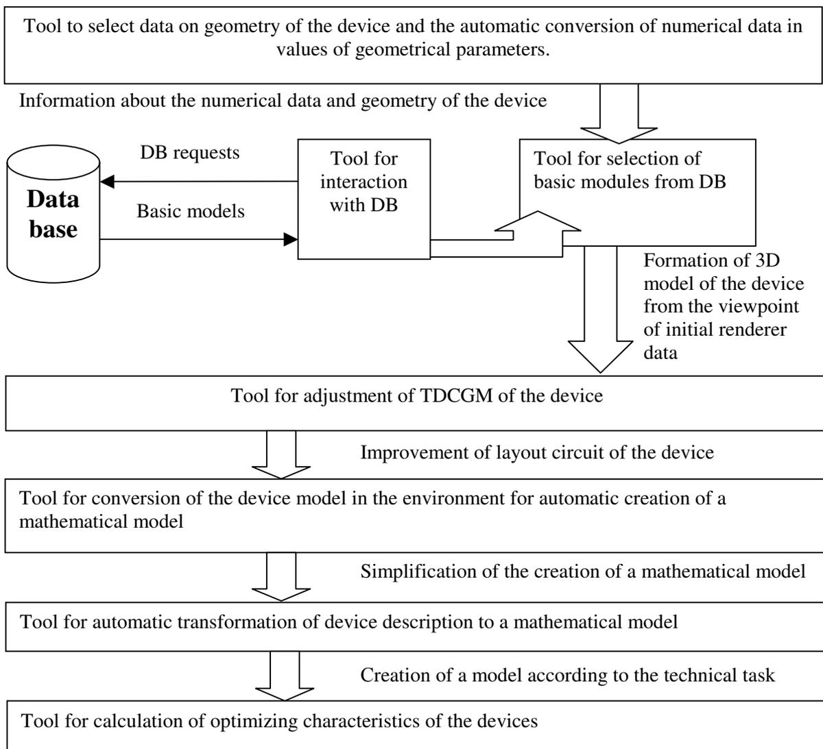
Fig. 1. Construction TCGM and optimizing the parameters of the simulated equipment
